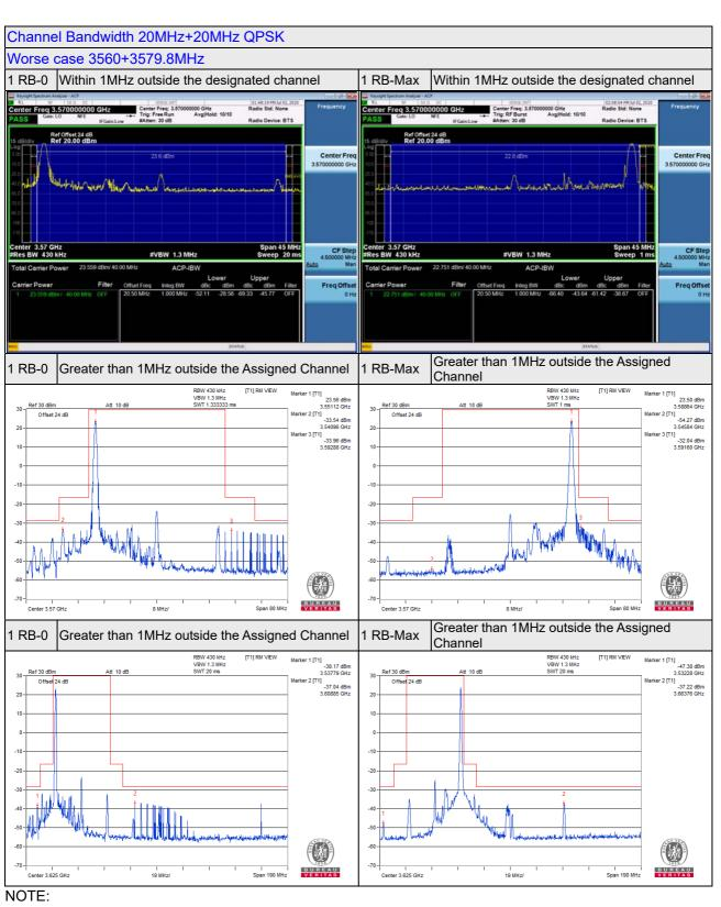
1MHz outside of designated channel needs to reduce the limit, When measured RBW less than 1MHz. Within 1-10MHz above the Assigned channel Limit is -13+10\*Log(430kHz/1MHz) = -16.66 dBm Within 1-10MHz below the Assigned channel Limit is -13+10\*Log(430kHz/1MHz) = -16.66 dBm 10MHz above the Assigned channel Limit is -25+10\*Log(430kHz/1MHz) = -28.66 dBm 10MHz below the Assigned channel Limit is -25+10\*Log(430kHz/1MHz) = -28.66 dBm
