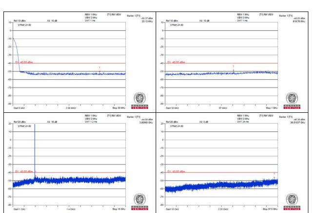
Note: The signal of 9kHz is IF signal from test instrument.
