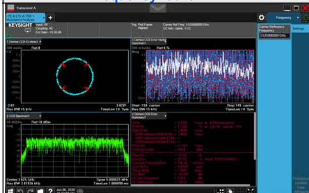
LTE 64QAM / Channel Bandwidth: 5MHz / Frequency: 3625 MHz
