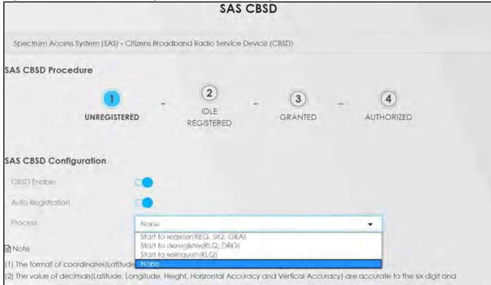
Figure 140 Network Setting &gt; SAS CBSD &gt; Unregistered
