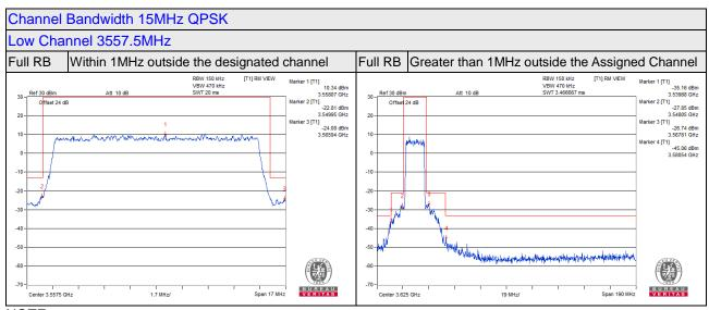
1MHz outside of designated channel needs to reduce the limit, When measured RBW less than 1MHz. Within 1- B MHz above the Assigned channel Limit is -13+10\*Log(150kHz/1MHz) = -21.24 dBm Within 1- B MHz below the Assigned channel Limit is -13+10\*Log(150kHz/1MHz) = -21.24 dBm B MHz above the Assigned channel Limit is -25+10\*Log(150kHz/1MHz) = -33.24 dBm B MHz below the Assigned channel Limit is -25+10\*Log(150kHz/1MHz) = -33.24 dBm
