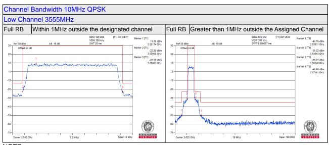
1MHz outside of designated channel needs to reduce the limit, When measured RBW less than 1MHz. Within 1- B MHz above the Assigned channel Limit is -13+10\*Log(100kHz/1MHz) = -23 dBm Within 1- B MHz below the Assigned channel Limit is -13+10\*Log(100kHz/1MHz) = -23 dBm B MHz above the Assigned channel Limit is -25+10\*Log(100kHz/1MHz) = -35 dBm B MHz below the Assigned channel Limit is -25+10\*Log(100kHz/1MHz) = -35 dBm
