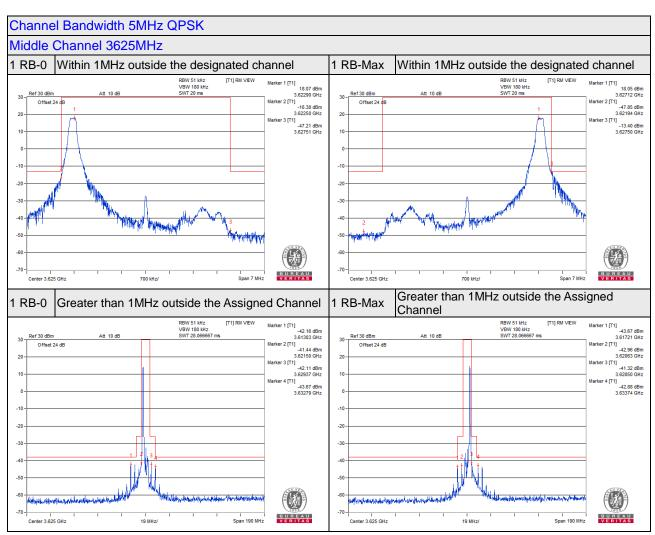
1MHz outside of designated channel needs to reduce the limit, When measured RBW less than 1MHz. Within 1- B MHz above the Assigned channel Limit is -13+10\*Log(51kHz/1MHz) = -25.92 dBm Within 1- B MHz below the Assigned channel Limit is -13+10\*Log(51kHz/1MHz) = -25.92 dBm B MHz above the Assigned channel Limit is -25+10\*Log(51kHz/1MHz) = -37.92 dBm B MHz below the Assigned channel Limit is -25+10\*Log(51kHz/1MHz) = -37.92 dBm
