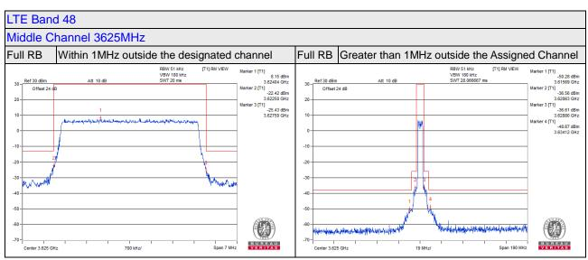
1MHz outside of designated channel needs to reduce the limit, When measured RBW less than 1MHz. Within 1- B MHz above the Assigned channel Limit is -13+10\*Log(51kHz/1MHz) = -25.92 dBm Within 1- B MHz below the Assigned channel Limit is -13+10\*Log(51kHz/1MHz) = -25.92 dBm B MHz above the Assigned channel Limit is -25+10\*Log(51kHz/1MHz) = -37.92 dBm B MHz below the Assigned channel Limit is -25+10\*Log(51kHz/1MHz) = -37.92 dBm
