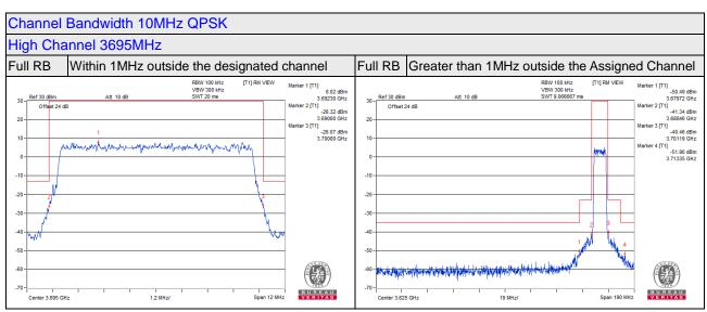
1MHz outside of designated channel needs to reduce the limit, When measured RBW less than 1MHz.
