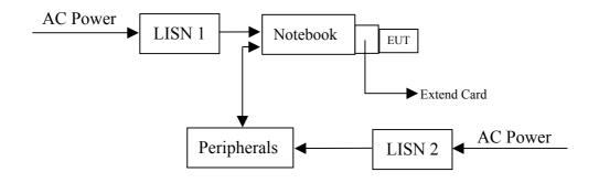
The EUT are connected to the main power through a line impedance stabilization network (LISN). This provides a 50 ohm/50uH coupling impedance for the measuring equipment. The peripheral devices are also connected to the main power through a LISN that provides a 500hm/50uH coupling impedance with 500hm termination.
