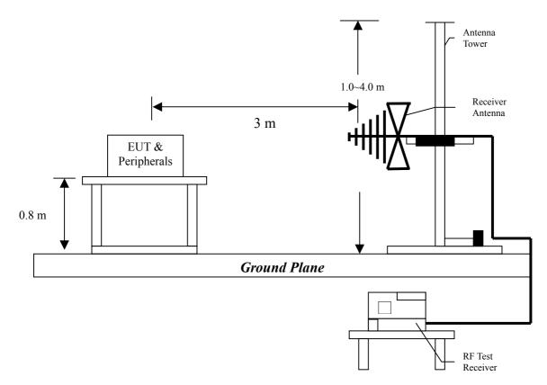
Radiated emissions were invested cover the frequency range from 30MHz to 1000MHz using a receiver RBW of 120kHz record QP reading, and the frequency over 1GHz using a spectrum analyzer RBW of 1MHz and 10Hz VBW record Average reading. (15.209 paragraph), the Peak reading (1MHz RBW/VBW) recorded also on the report.
