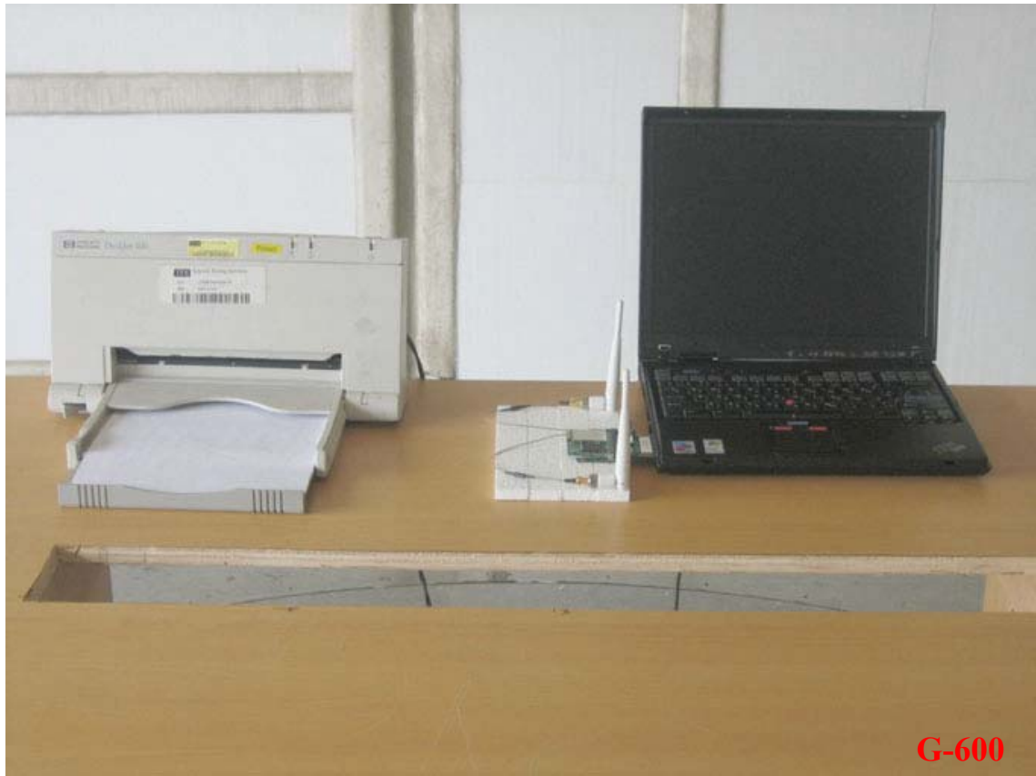
Photo 1: Radiated Emission Test set-up photo
