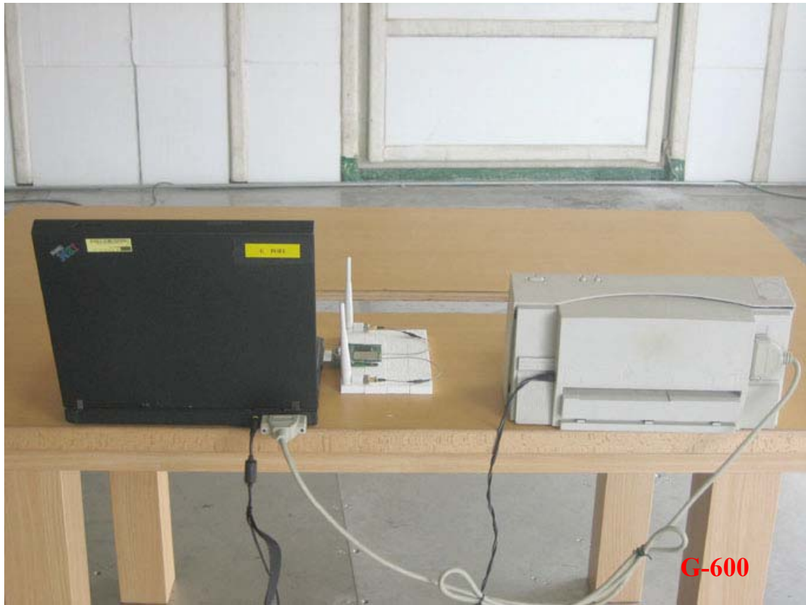
Photo 2: Radiated Emission Test set-up photo
