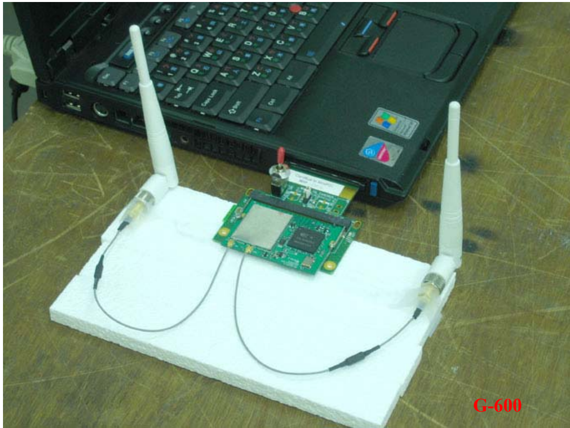
Photo 3: Conducted Emission Test Set-up photo
