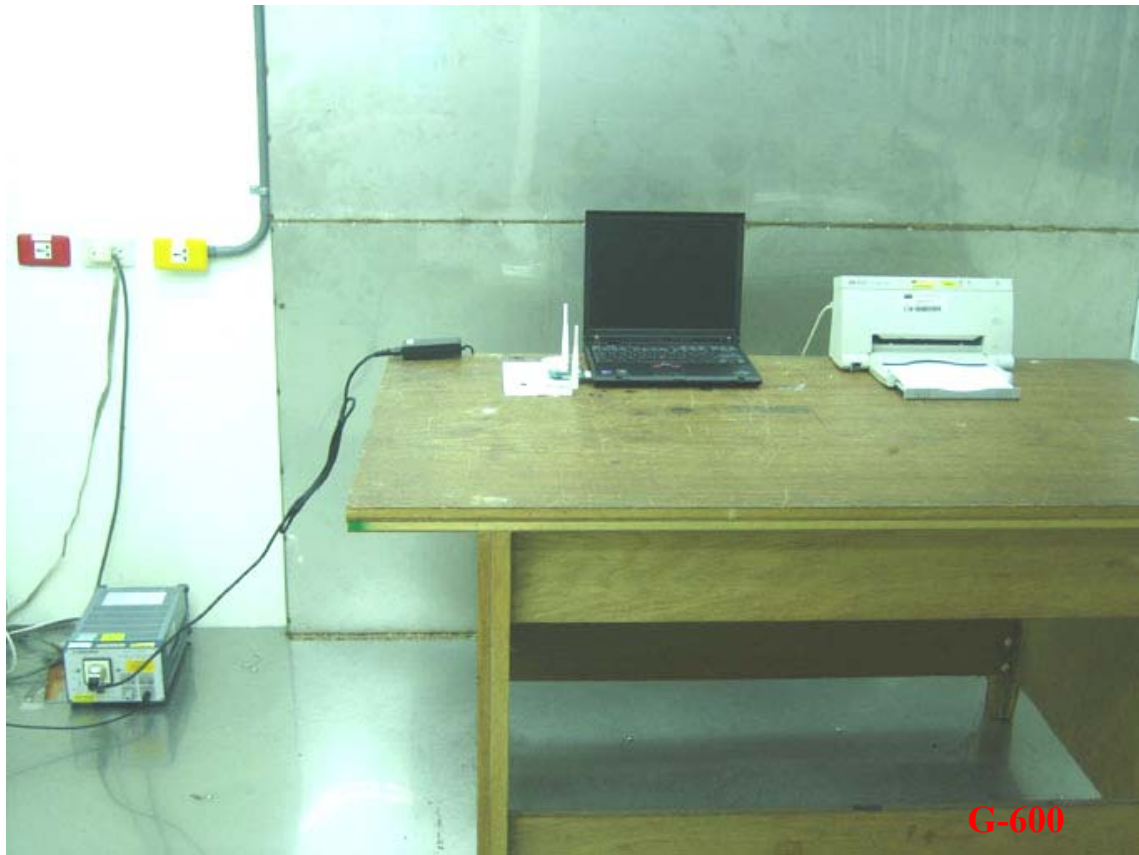
Photo 1: Conducted Emission Test Set-up photo
