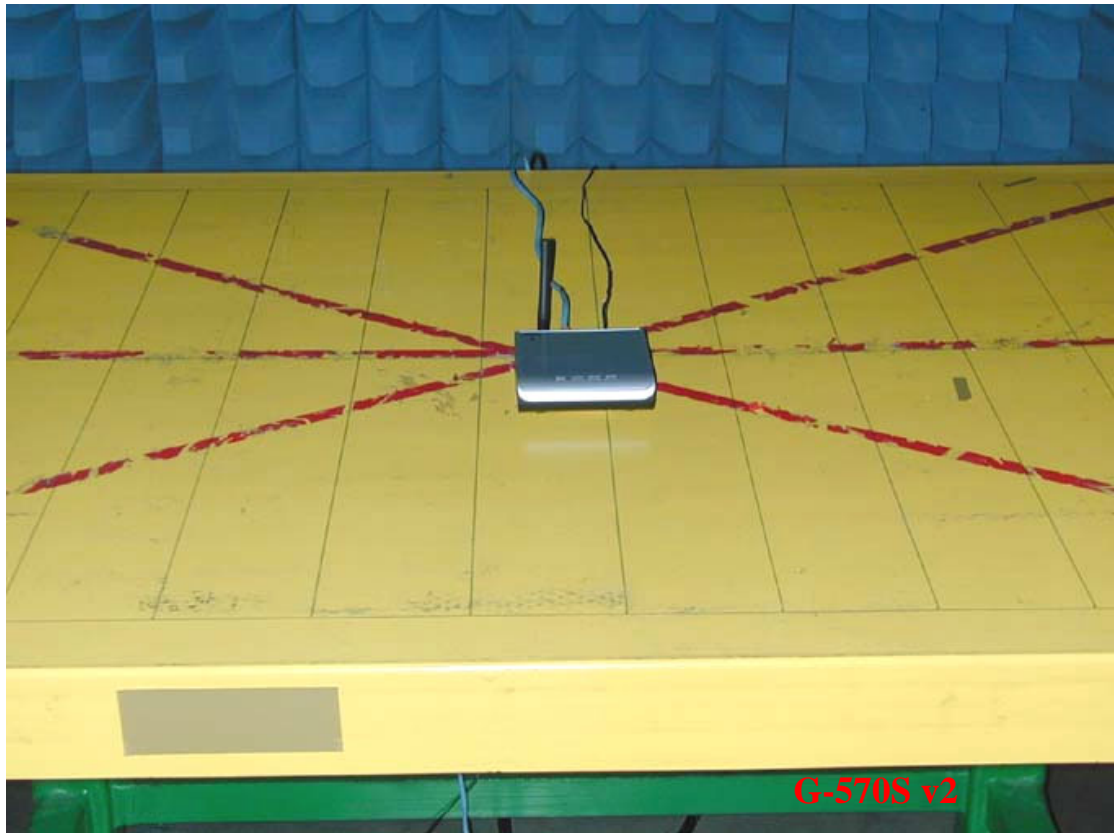
Photo 1: Radiated Emission Test set-up photo
