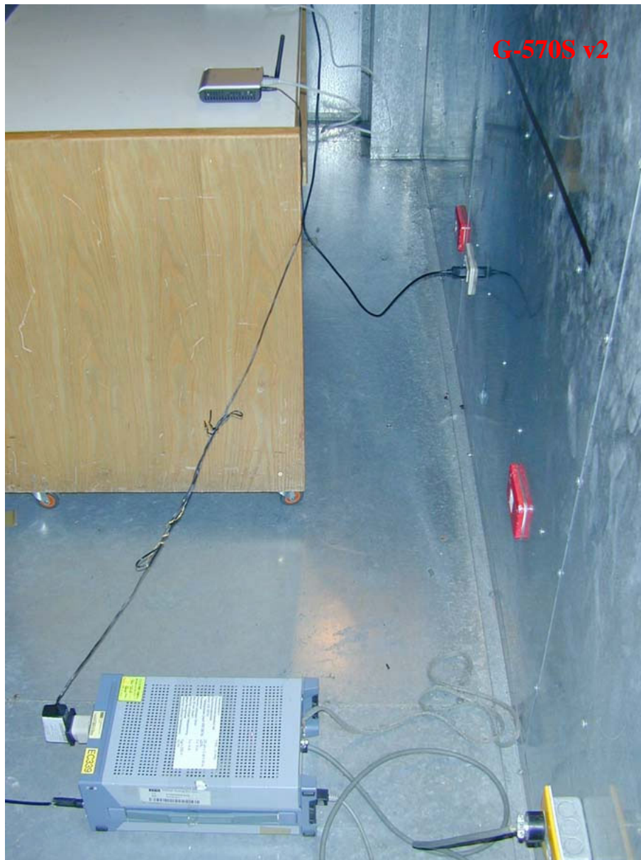
Photo 2: Conducted Emission Test Set-up photo
