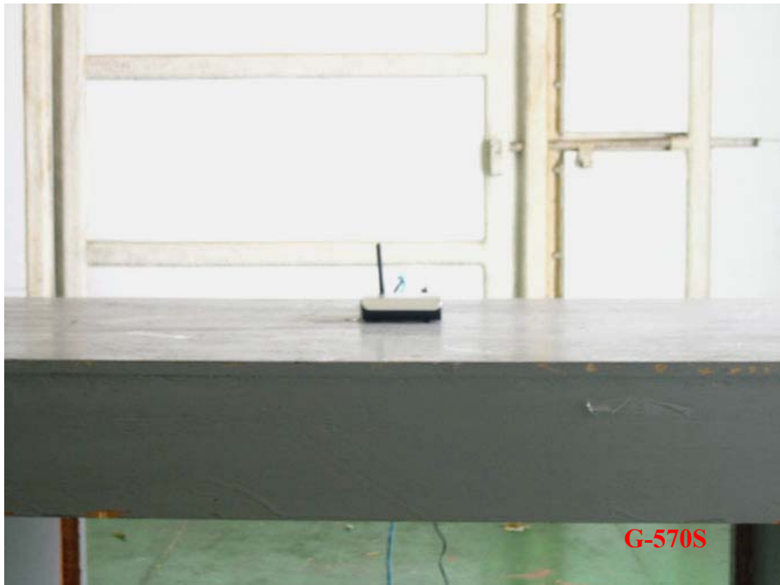
Photo 1: Radiated Emission Test set-up photo
