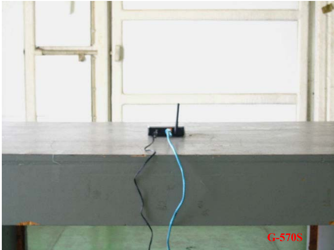
Photo 2: Radiated Emission Test set-up photo
