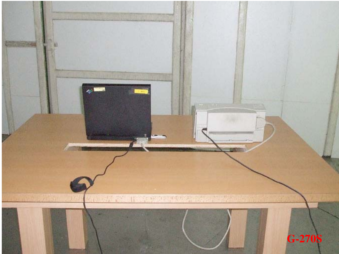
Photo 2: Radiated Emission Test set-up photo
