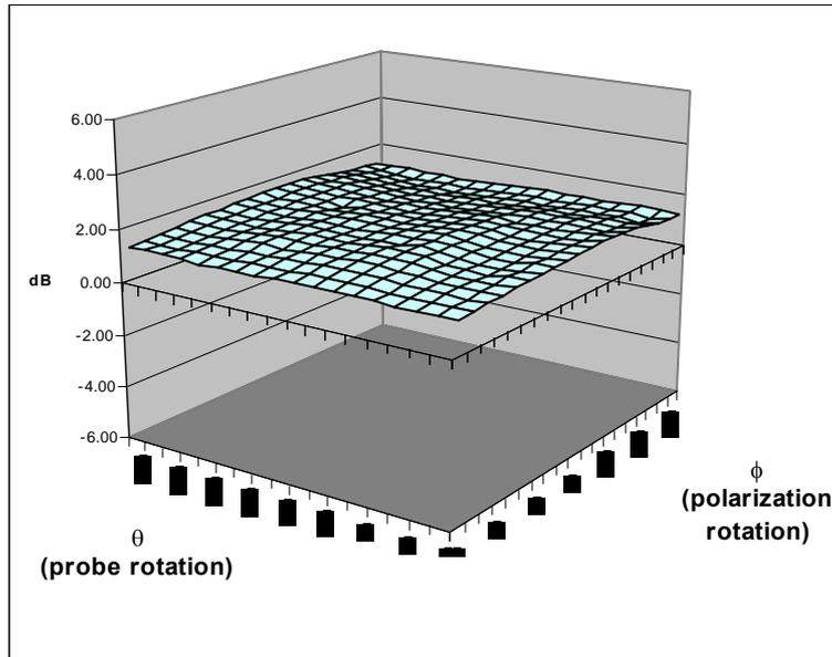
**Surface Isotropy diagram of IXP-050 Probe S/N 0136 at 900MHz after VPM**
