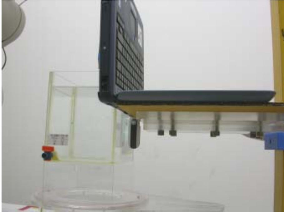
**Figure 9: EUT bottom to phantom, 0 mm separation-Zoom in**
