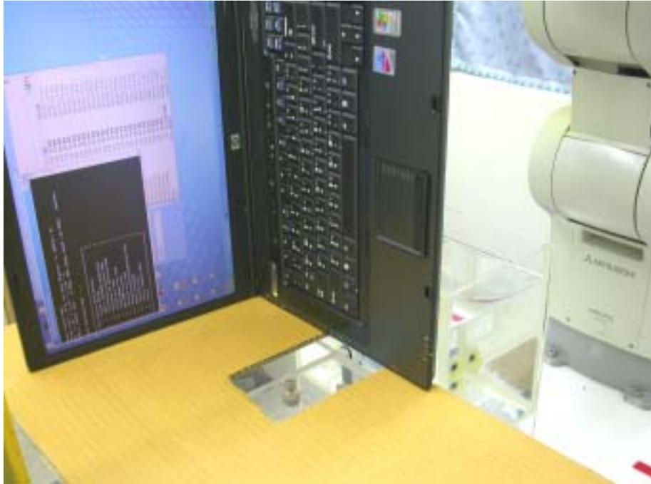
**Figure 15: EUT bottom to phantom, 0 mm separation-Zoom in**
