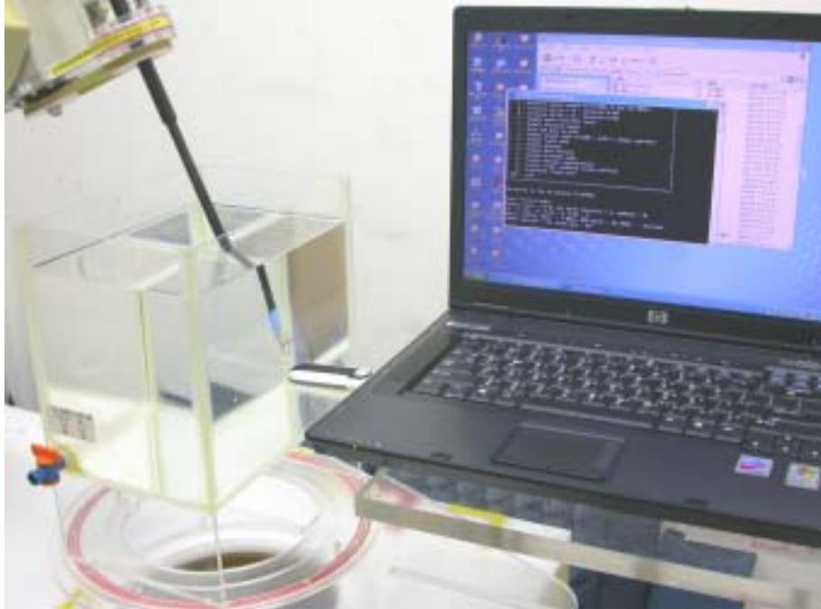
**Figure 17: EUT perpendicular to phantom, 0 mm separation-Zoom in**
