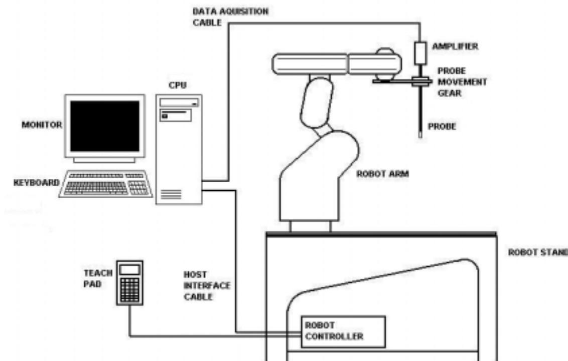
Figure 1: Schematic diagram of the SAR measurement system
