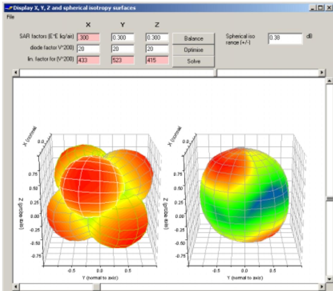
**Figure 3. Typical graphical representation of a probe's response to fields applied from each direction. The diagram on the left shows the individual response characteristics of each of the three channels and the diagram on the right shows the resulting probe sensitivity in each direction. The colour range in the figure images the lowest values as blue and the maximum values as red. For the probe S/N 0136, this range is (+/-) 0.24dB.**
