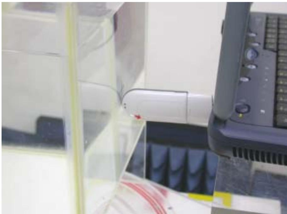
**SAR Measurement Test Setup**
