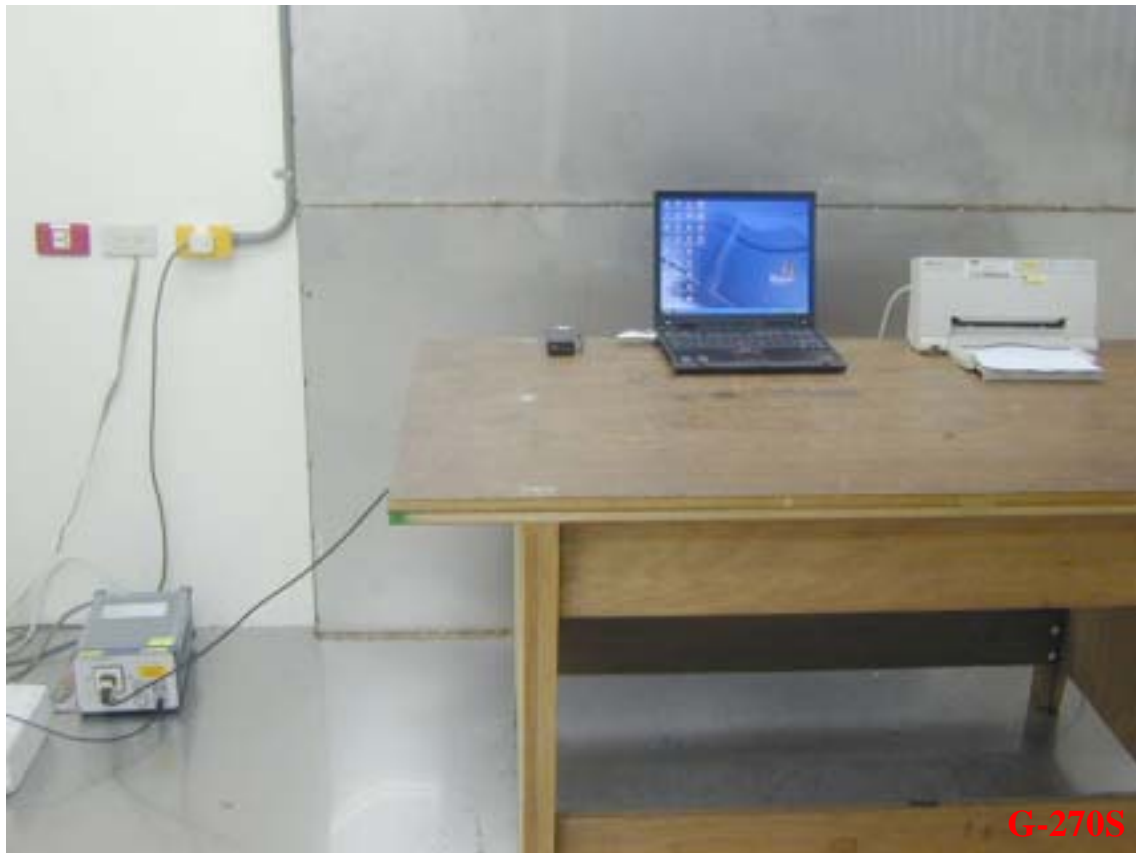
Photo 1: Conducted Emission Test set-up photo
