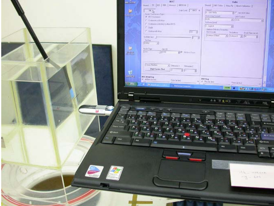
Figure 4: EUT perpendicular to phantom, 0 mm separation
