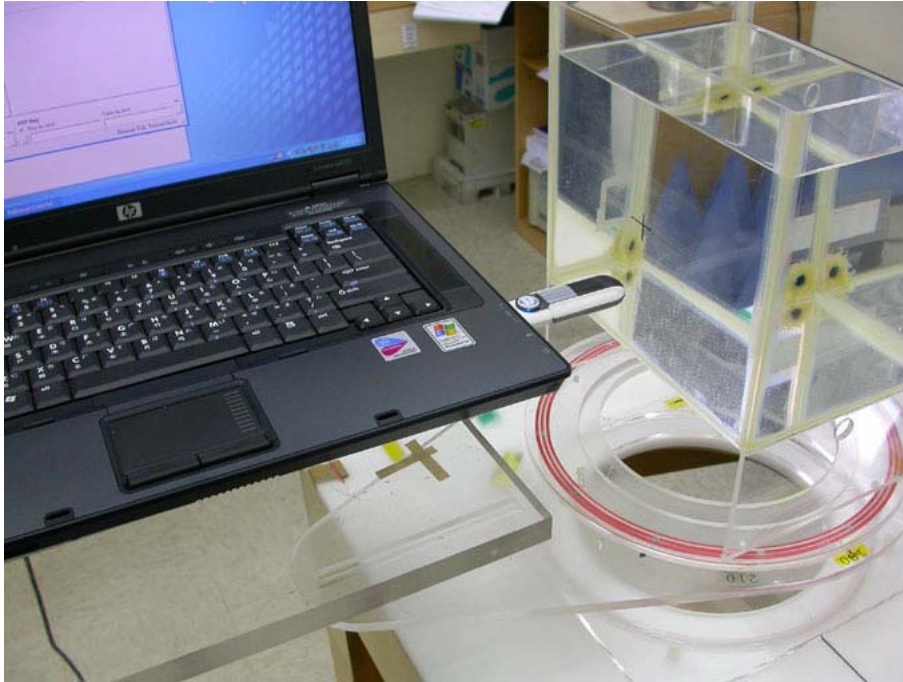
Figure 18: EUT perpendicular to phantom, 15 mm separation
