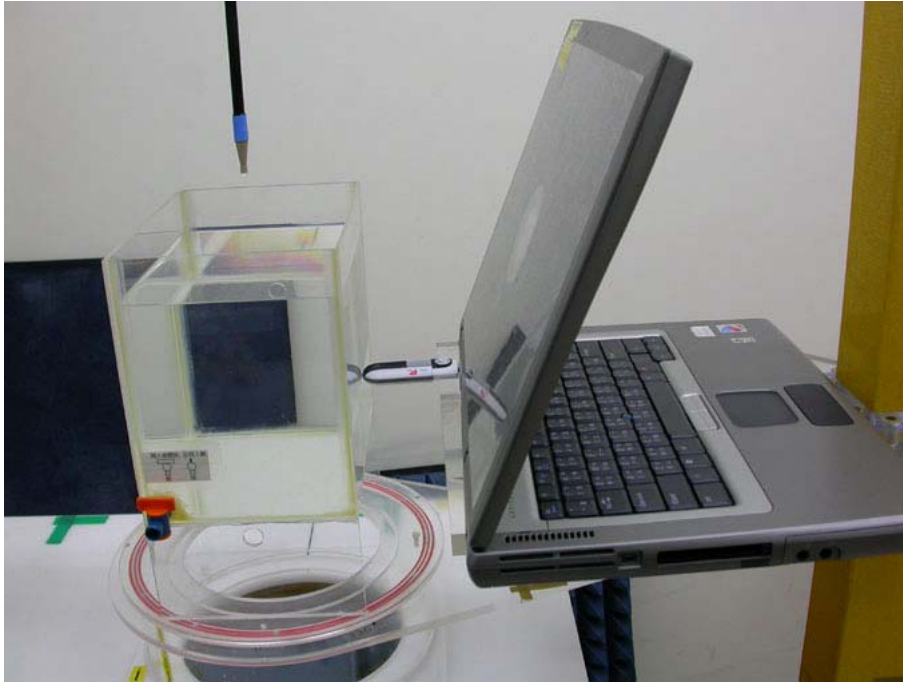
Figure 10: EUT perpendicular to phantom, 0 mm separation
