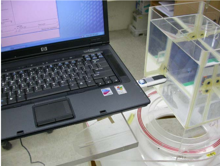
Figure 16: EUT perpendicular to phantom, 0 mm separation
