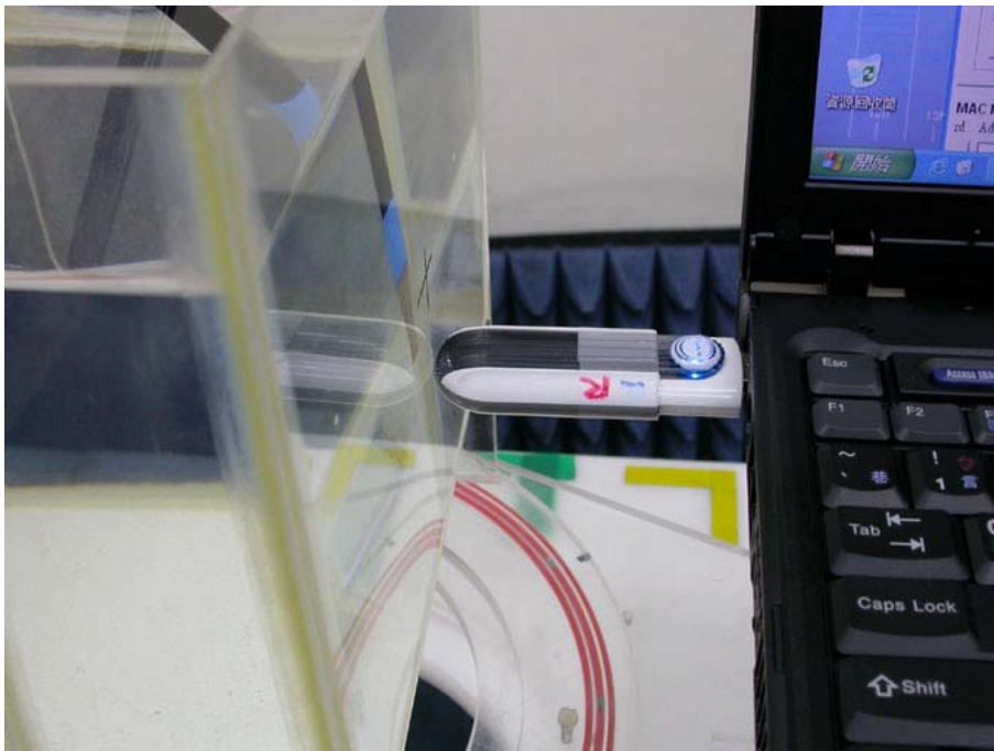
Figure 5: EUT perpendicular to phantom, 0 mm separation- Zoom In
