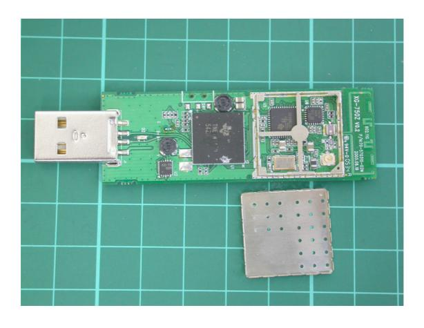
**Photo 4: Internal photo of EUT**
