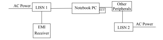
The EUT are connected to the main power through a line impedance stabilization network (LISN). This provides a 50 ohm/50uH coupling impedance for the measuring equipment. The peripheral devices are also connected to the main power through a LISN that provides a 50ohm/50uH coupling impedance with 50ohm termination.
