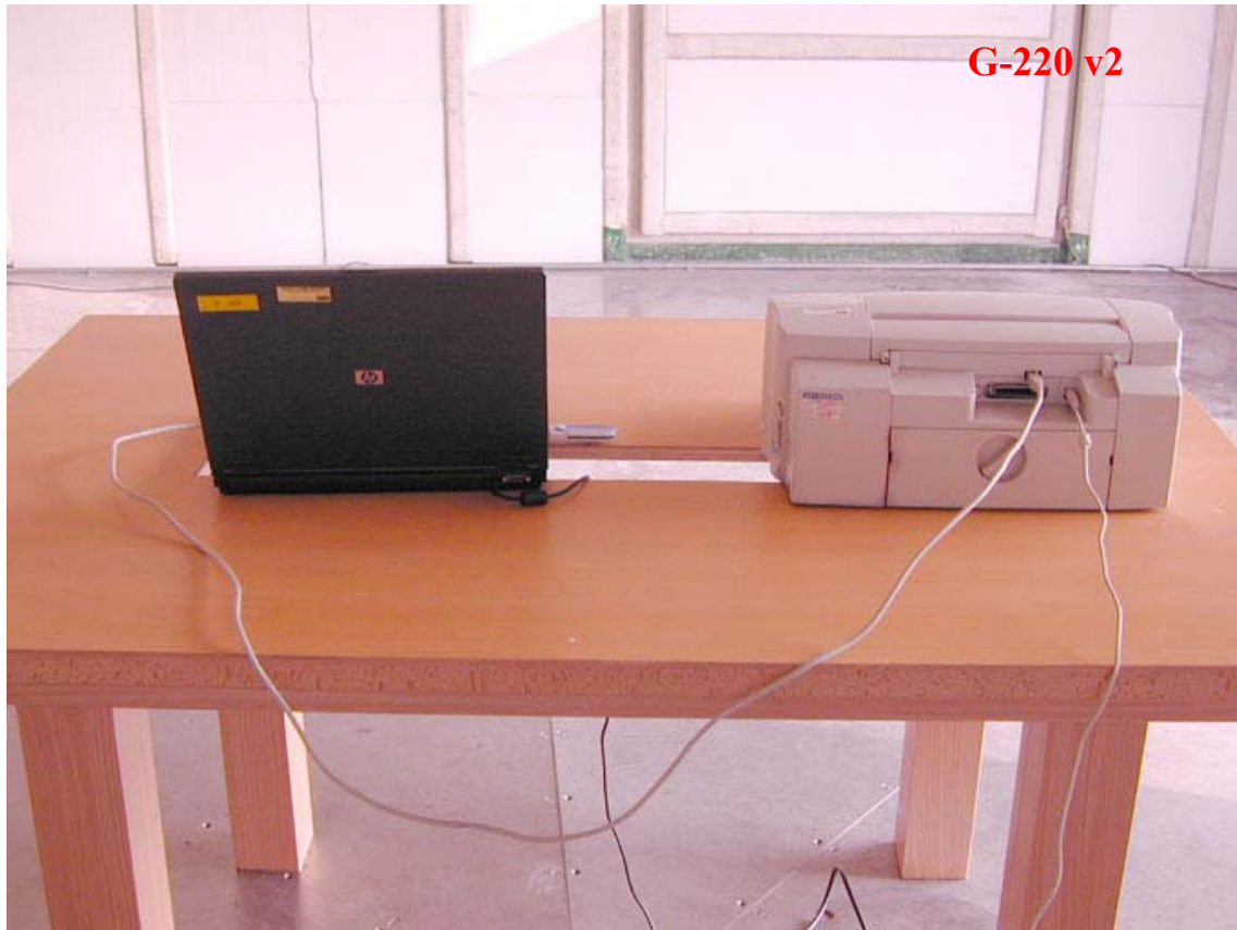
Photo 2: Radiated Emission Test set-up photo
