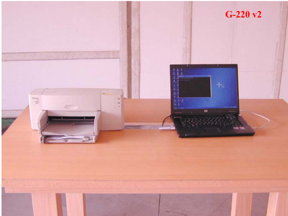
Photo 1: Radiated Emission Test set-up photo
