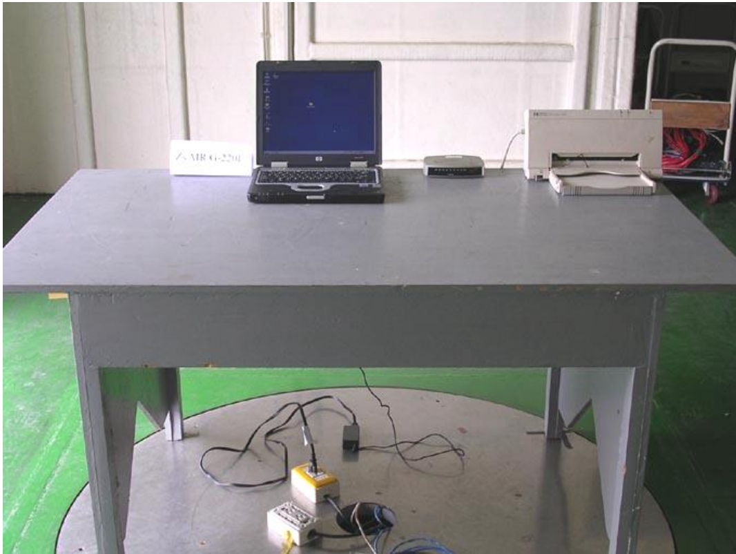
Photo 1: Radiated Emission Test set-up photo
