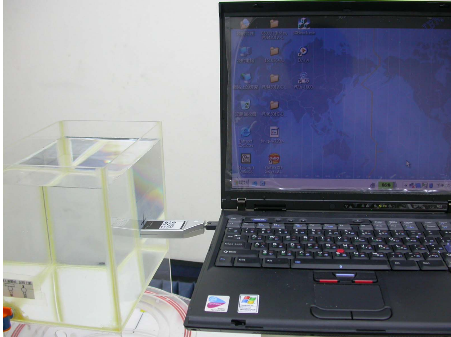
Figure 6: EUT perpendicular to phantom, 0 mm separation (with EUT lie down)
