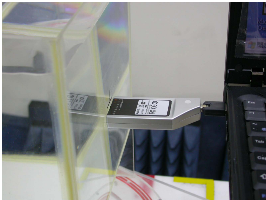
Figure 7: EUT perpendicular to phantom, 0 mm separation (with EUT lie down) - Zoom In
