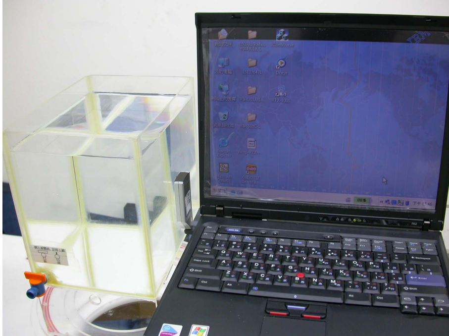
Figure 8: EUT perpendicular to phantom, 0 mm separation (with EUT stand)
