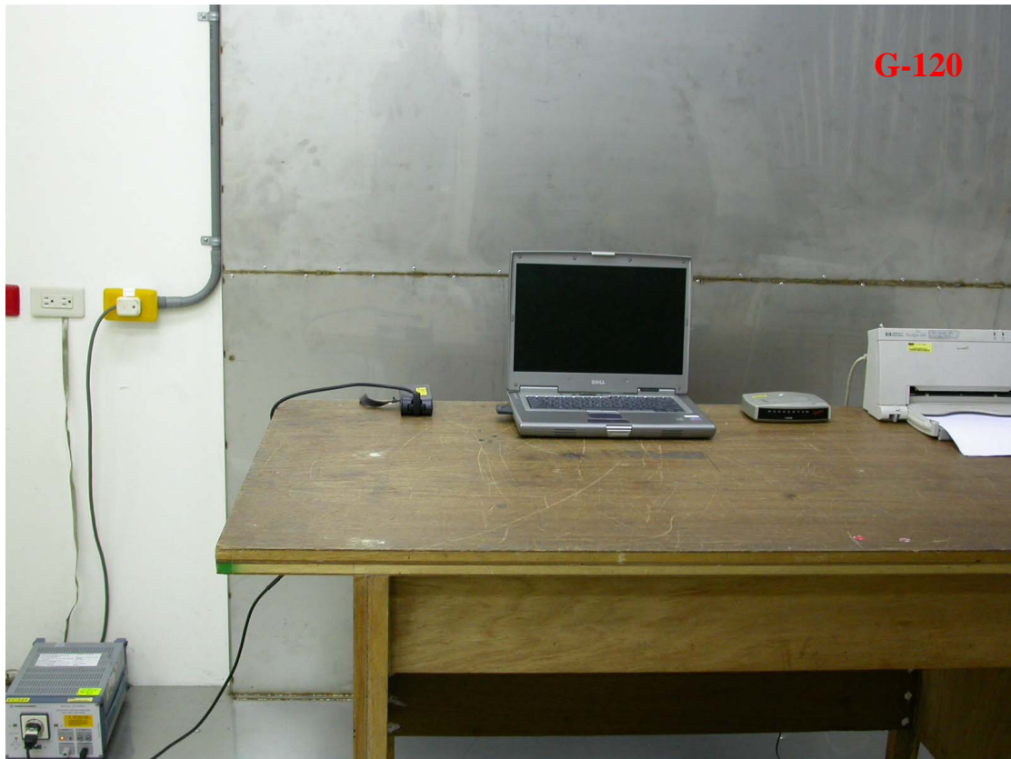
Photo 1: Conducted Emission Test Set-up photo
