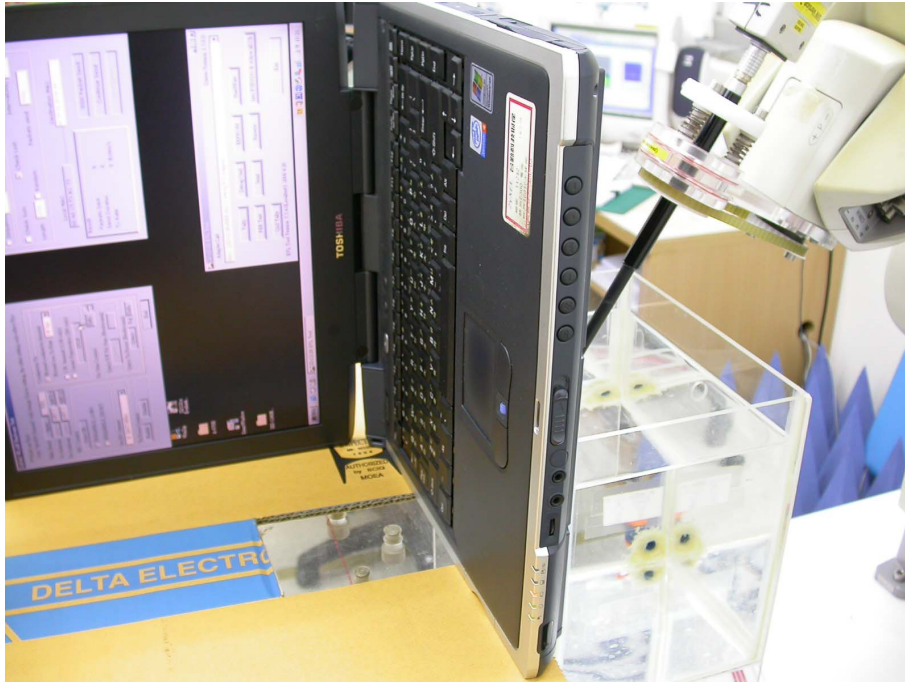
Figure 14: EUT bottom to phantom, 0 mm separation
