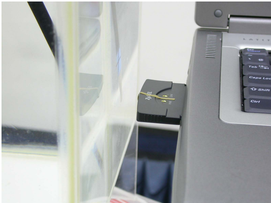
Figure 7: EUT perpendicular to phantom, 15 mm separation-Zoom in
