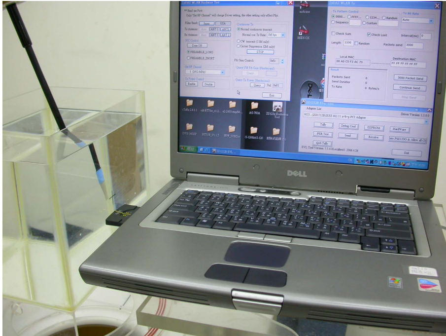
Figure 4: EUT perpendicular to phantom, 0 mm separation
