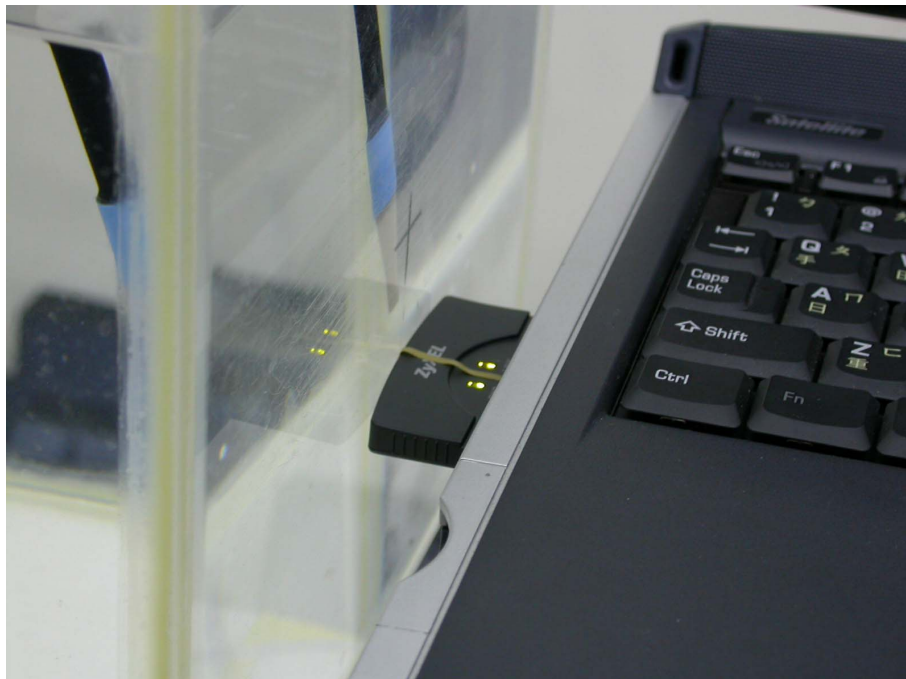
Figure 17: EUT perpendicular to phantom, 0 mm separation-Zoom in
