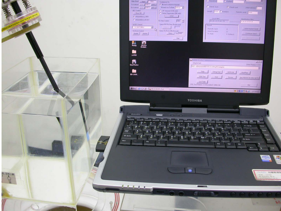
Figure 18: EUT perpendicular to phantom, 15 mm separation
