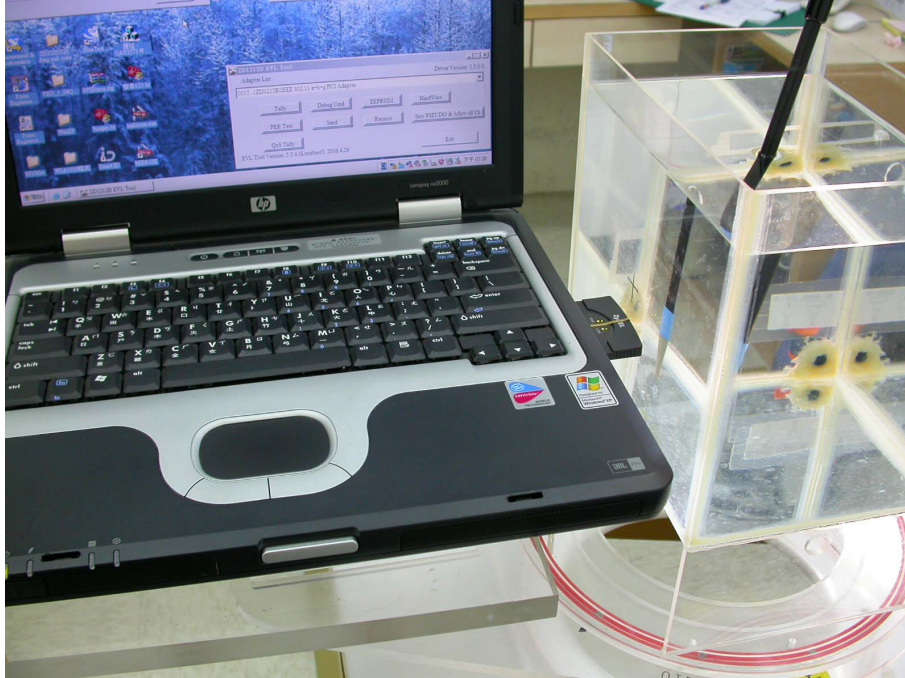
Figure 10: EUT perpendicular to phantom, 0 mm separation
