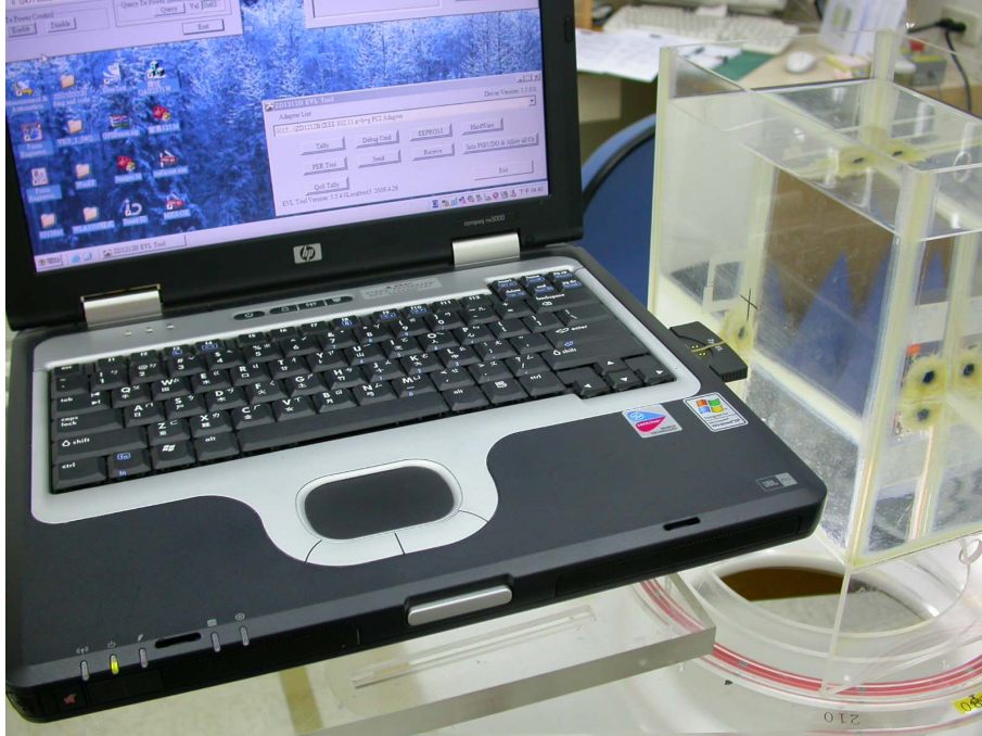
Figure 12: EUT perpendicular to phantom, 15 mm separation
