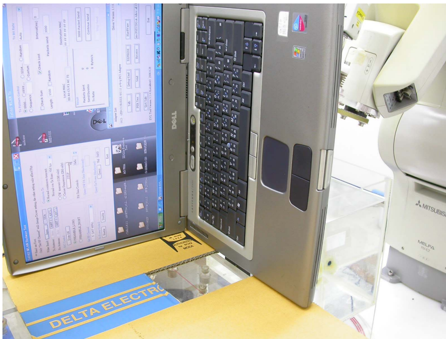
Figure 2: EUT bottom to phantom, 0 mm separation
