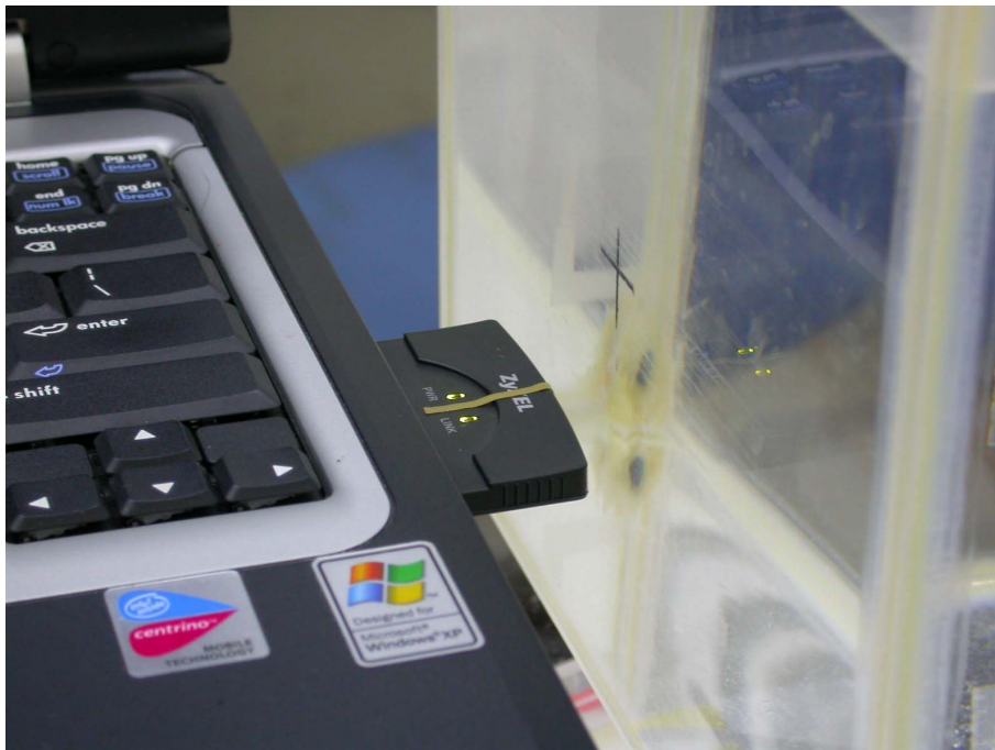
Figure 13: EUT perpendicular to phantom, 15 mm separation-Zoom in
