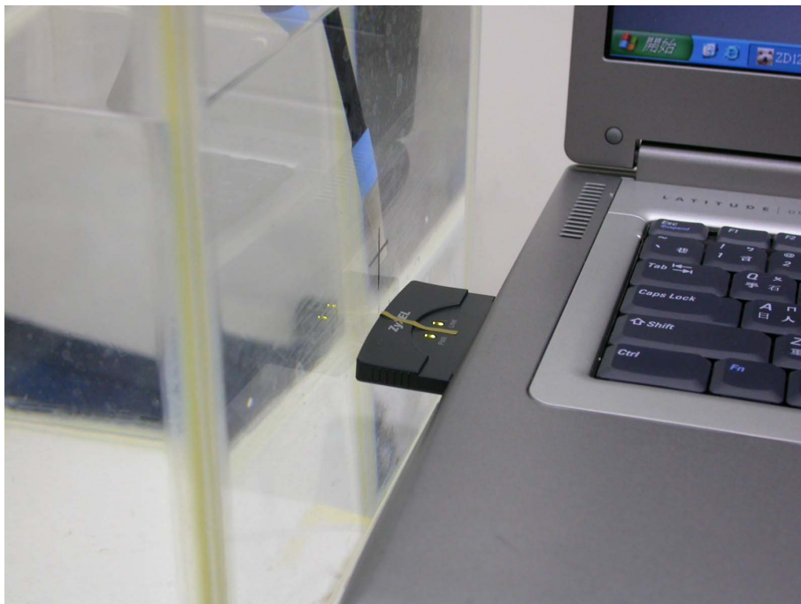
Figure 5: EUT perpendicular to phantom, 0 mm separation-Zoom in
