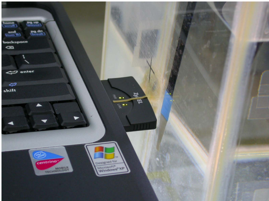
Figure 11: EUT perpendicular to phantom, 0 mm separation-Zoom in
