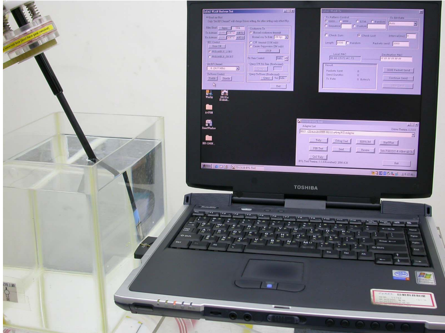
Figure 16: EUT perpendicular to phantom, 0 mm separation
