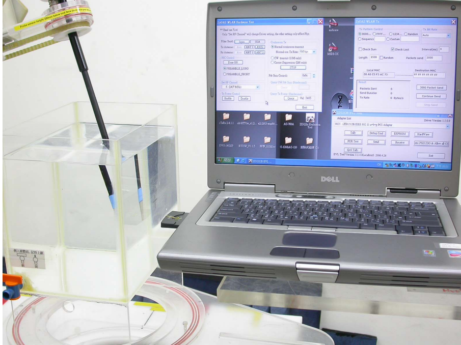
Figure 6: EUT perpendicular to phantom, 15 mm separation
