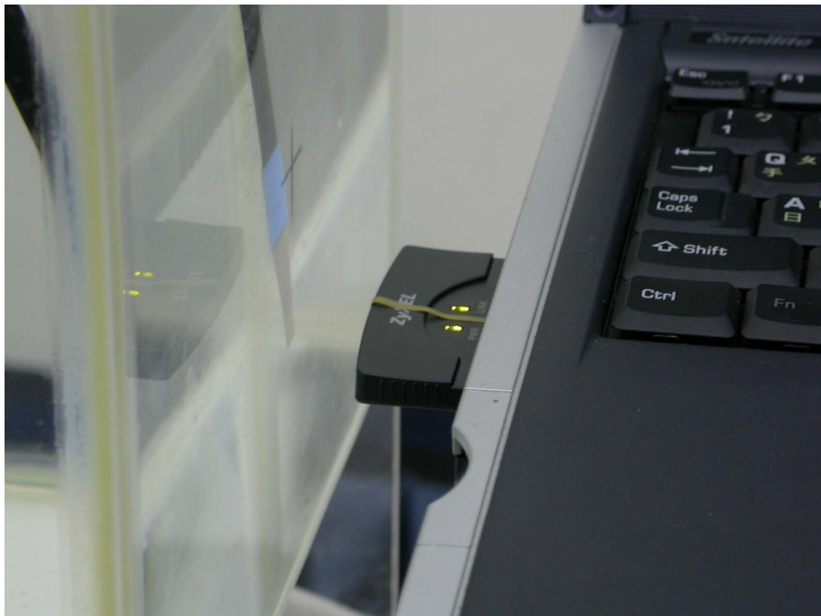
Figure 19: EUT perpendicular to phantom, 15 mm separation-Zoom in
