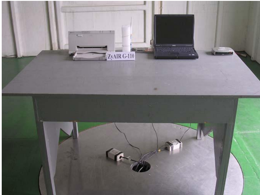
Photo 1: Radiated spurious test set-up photo (front)
