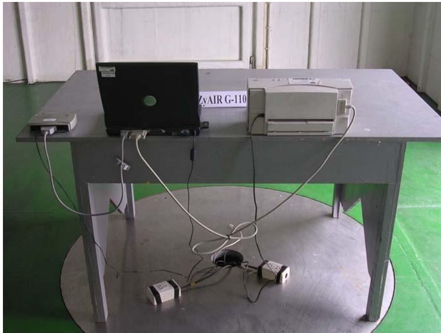
Photo 4: Radiated spurious test set-up photo (rear)
