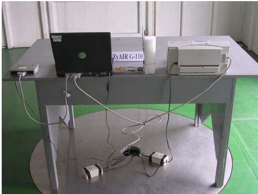
Photo 2: Radiated spurious test set-up photo (rear)
