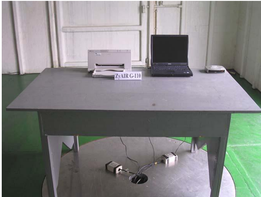
Photo 3: Radiated spurious test set-up photo (front)
