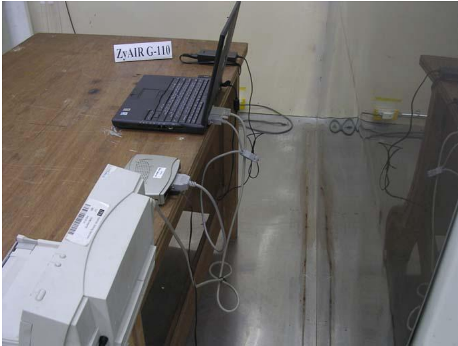
Photo 4: Conducted Test Set-up photo (rear)
