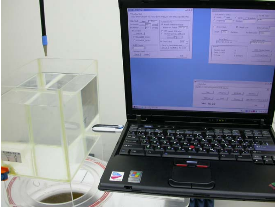
Figure 12: EUT perpendicular to phantom, 15 mm separation
