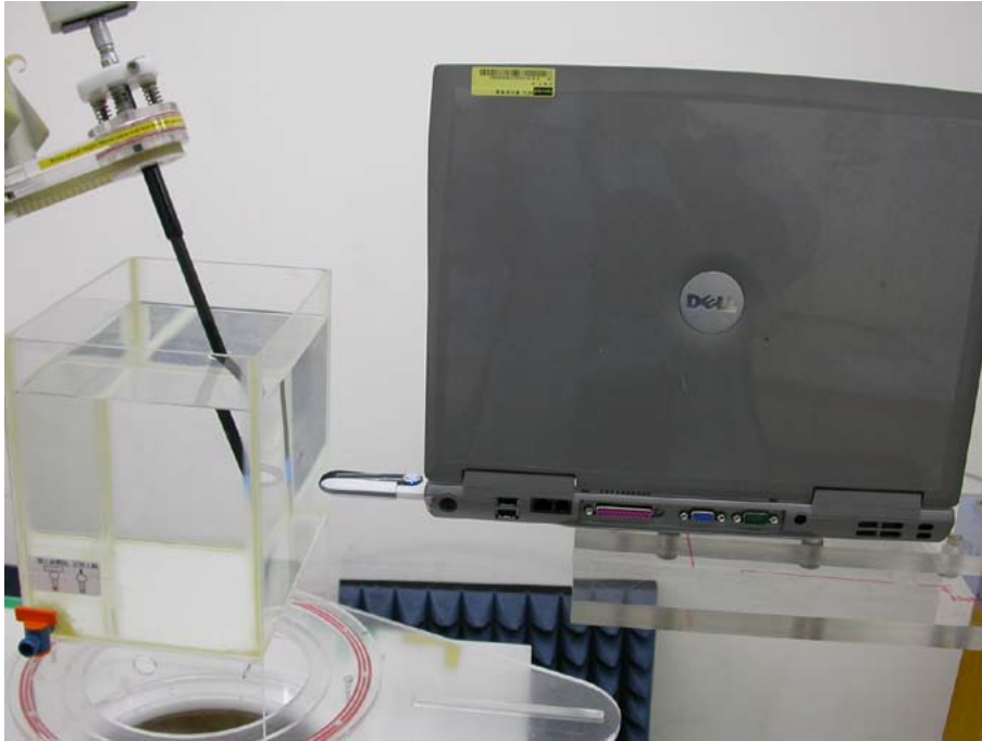
Figure 6: EUT perpendicular to phantom, 15 mm separation
