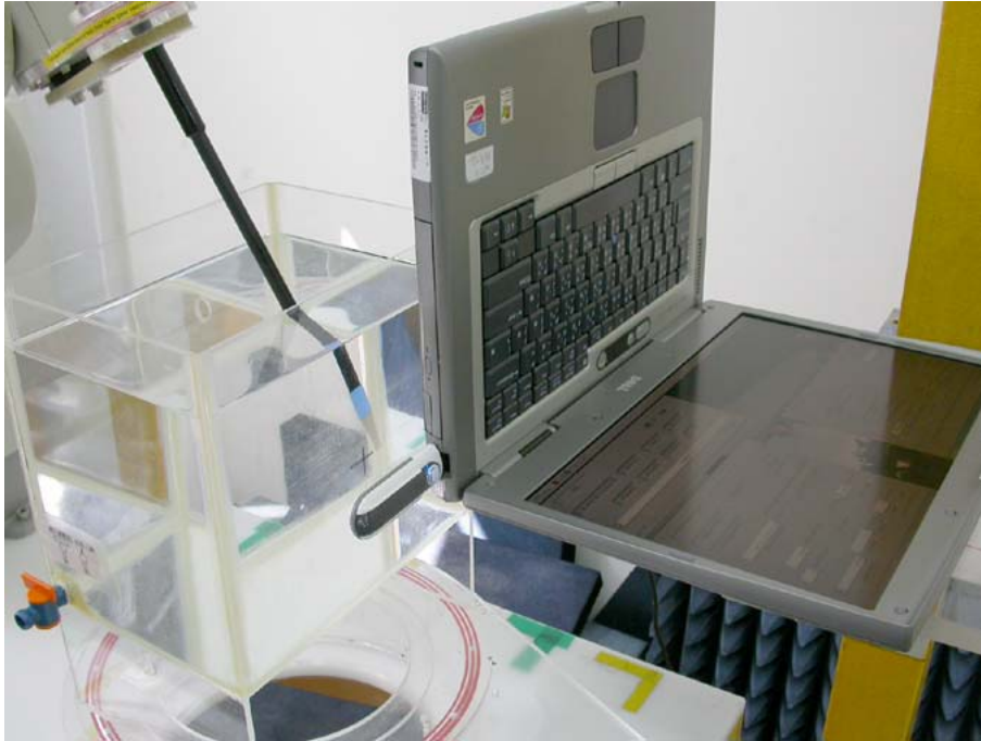
Figure 2: Bottom side of Laptop facing phantom touching
