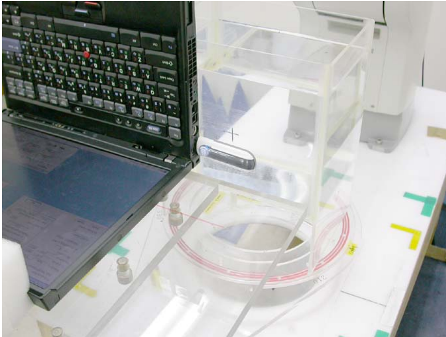
Figure 8: Bottom side of Laptop facing phantom touching
