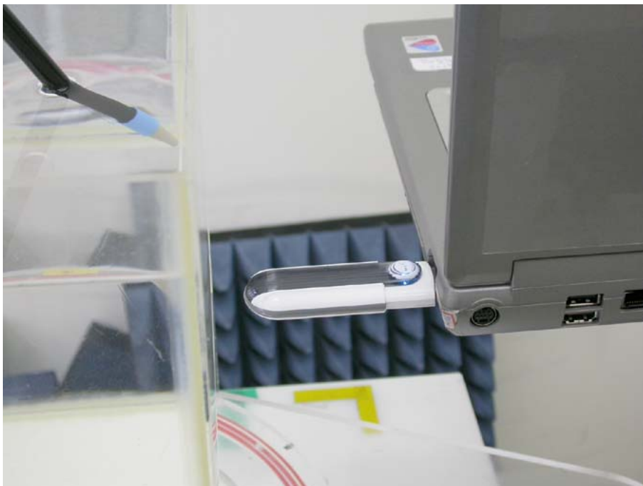
Figure 7: EUT perpendicular to phantom, 15 mm separation- Zoom In
