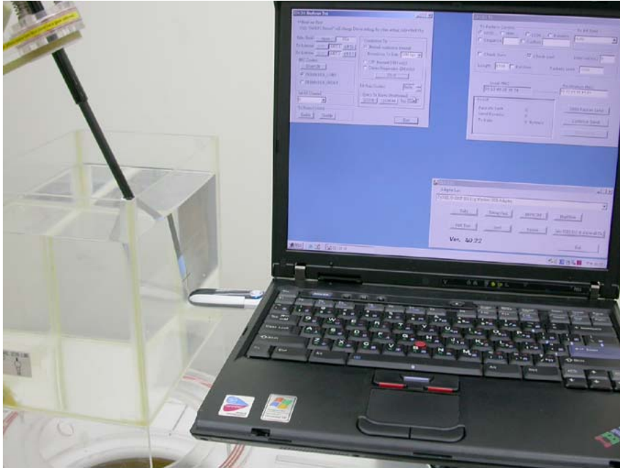
Figure 10: EUT perpendicular to phantom, 0 mm separation
