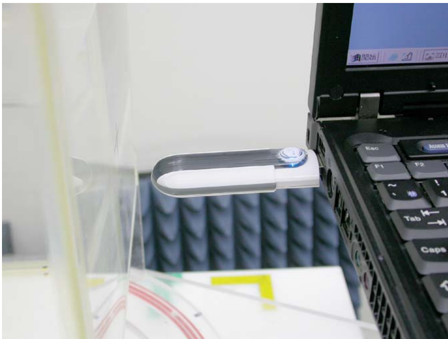
Figure 13: EUT perpendicular to phantom, 15 mm separation- Zoom In
