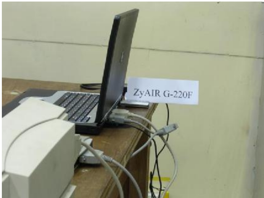
Photo 2: Conducted Emission Test Set-up photo
