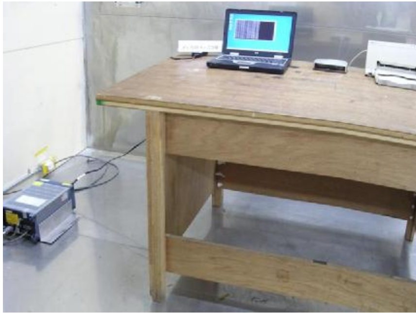
Photo 2: Conducted Emission Test Set-up photo
