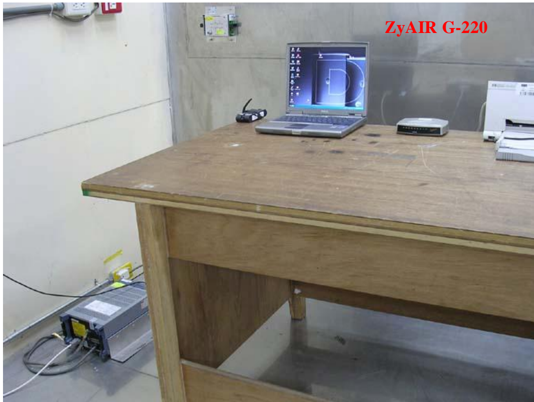
Photo 1: Conducted Emission Test Set-up photo
