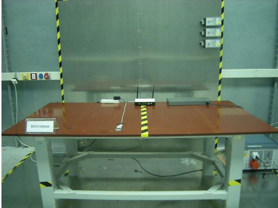
Front View of Conducted Emission Test
