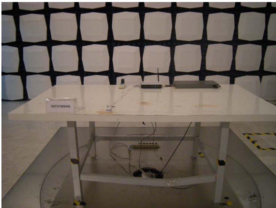
Front View of Radiated Emission Test
