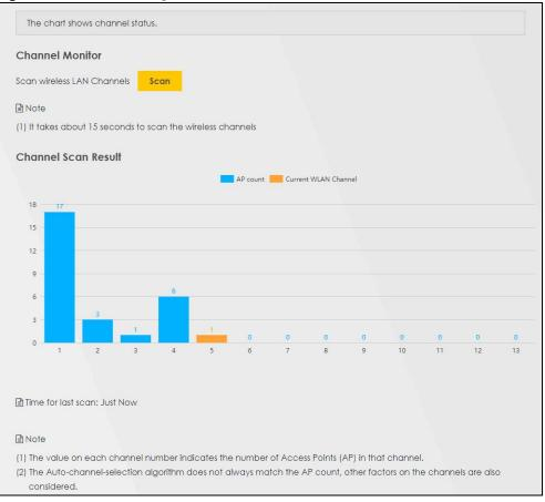
Figure 57 Network Setting > Wireless > Channel Status
