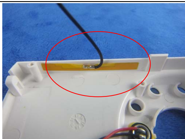
WiFi Antenna View
