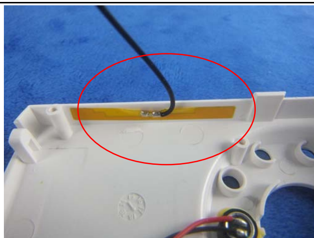
WiFi Antenna View
