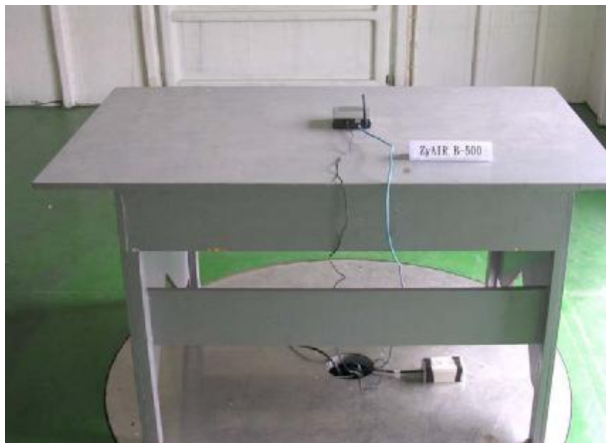
Photo 2: Radiated Emission Test Set-up (rear)
