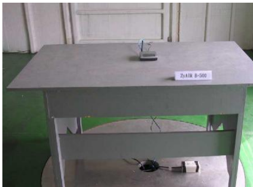
Photo 1: Radiated Emission Test Set-up (front)
