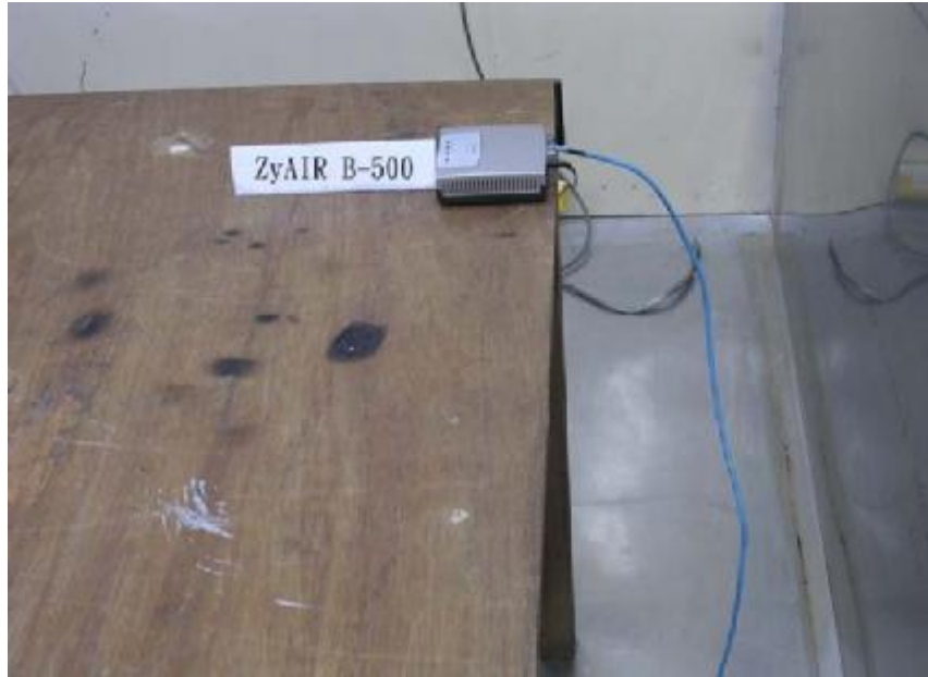
Photo 2: Conducted Emission Test Set-up (rear)
