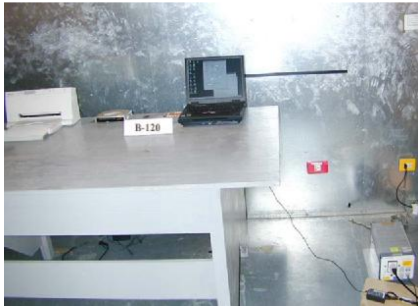
Photo 1: Conducted Test Set-up (front)
