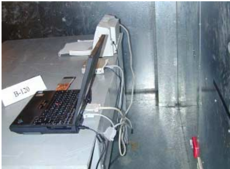
Photo 2: Conducted Test Set-up (rear)
