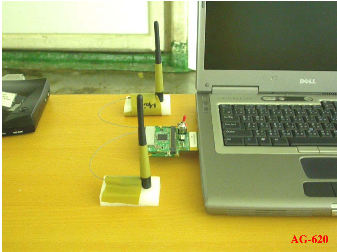
Photo 2: Radiated Emission Test set-up photo
