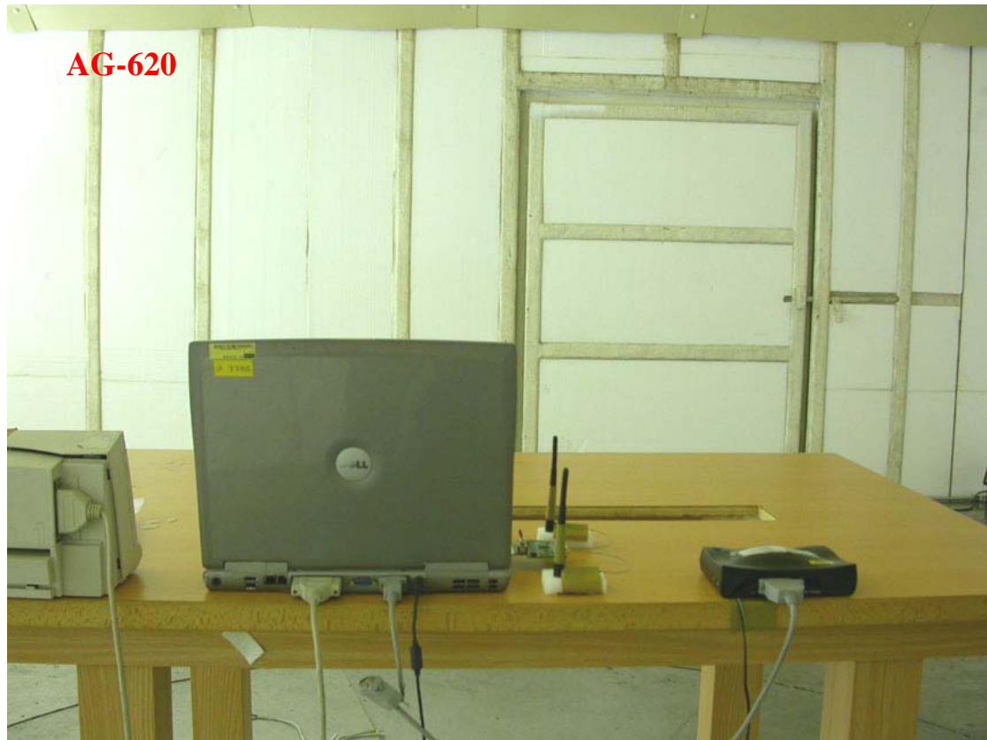
Photo 3: Radiated Emission Test set-up photo
