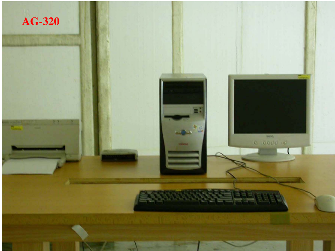
Photo 3: Radiated Emission Test set-up photo
