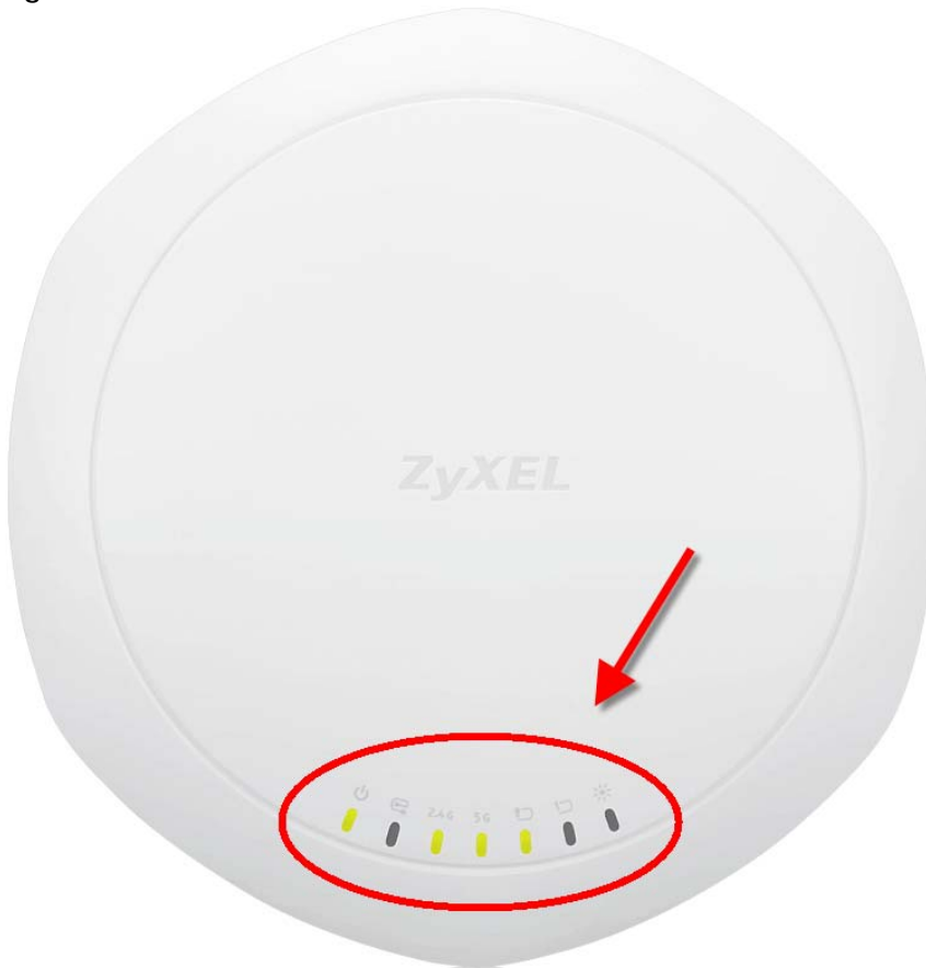
Figure 20 NWA1123-AC PRO LEDs
