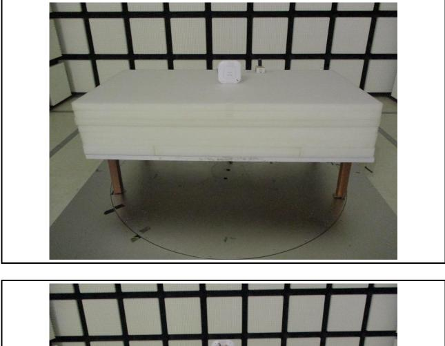
Radiated Emission Below 1GHz Test (Adapter Mode)
