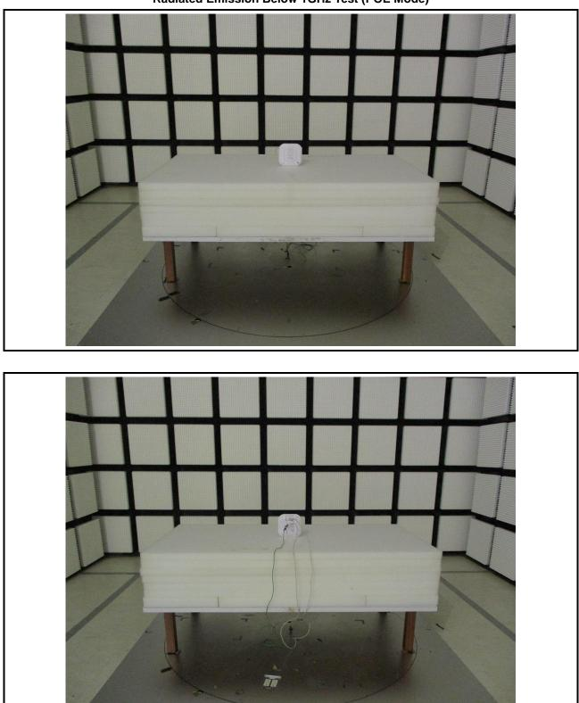
Radiated Emission Below 1GHz Test (POE Mode)
