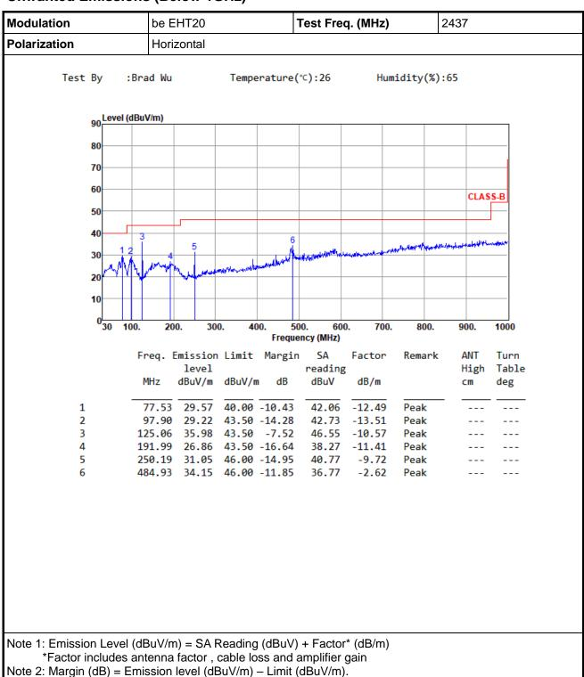
Note 3: All spurious emissions below 30MHz are more than 20 dB below the limit.
