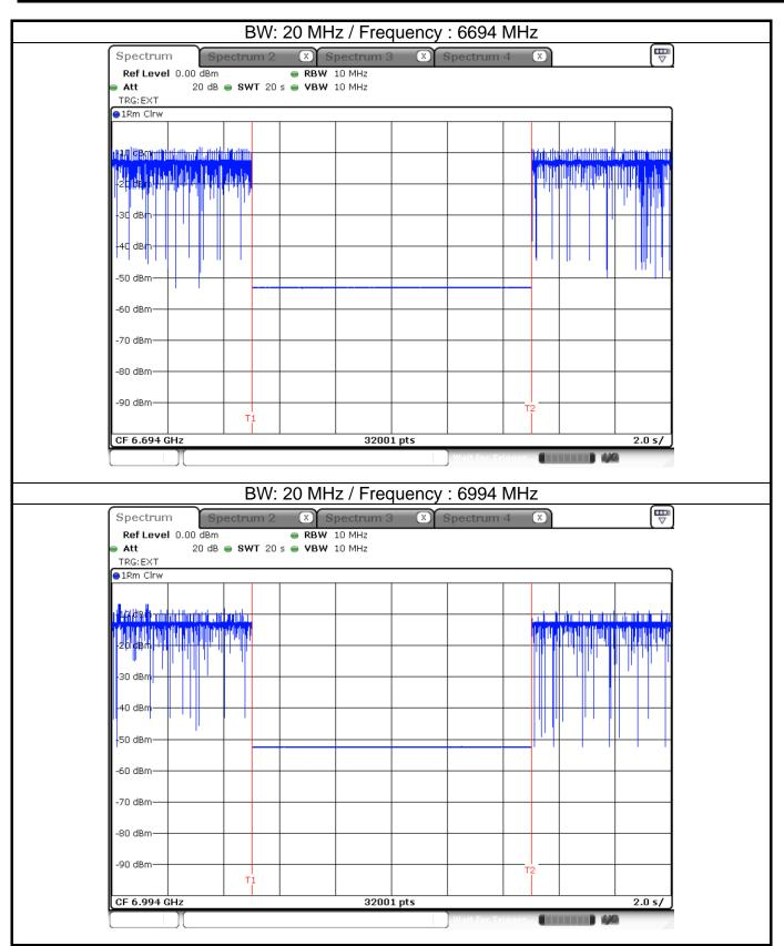
Note: T1: AWGN signal is injected, T2: AWGN signal is removed.
