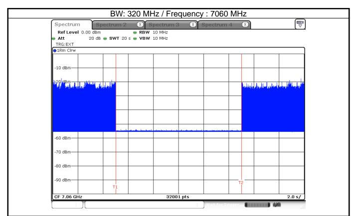
Note: T1: AWGN signal is injected, T2: AWGN signal is removed.
