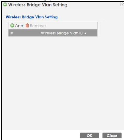
Figure 71 Configuration > Wireless > AP Management > Setup Wireless Bridge Vlan ID: Wireless Bridge Vlan Setting (for Zyxel Device with multiple Ethernet ports)
