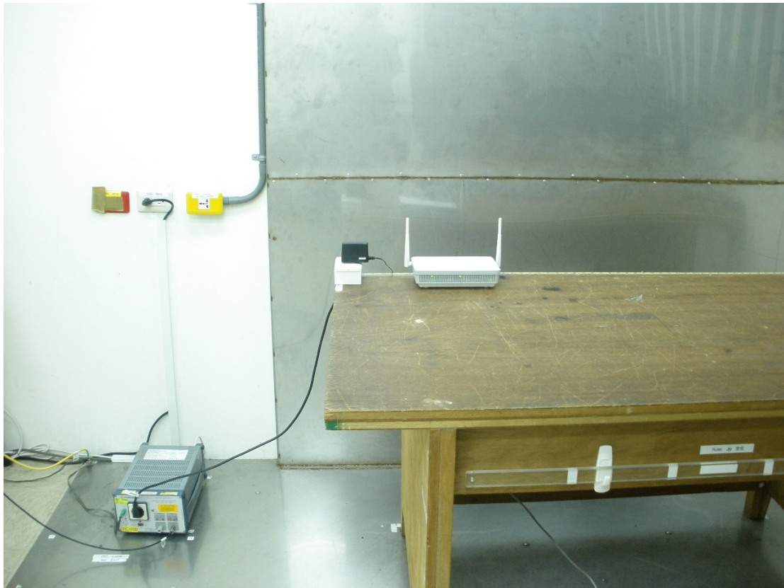
Photo 1: Conducted Emission Test Set-up photo
