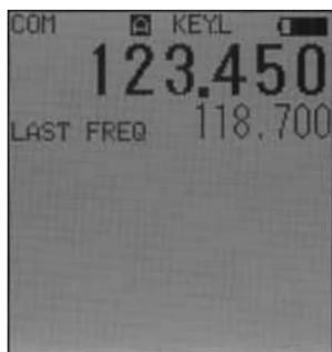
Key Lock is deactivated by holding the Clear key and pressing the Down key a second time. Key Lock only locks out the PJ2+ COM's keypad. The PTT and Light functions are not affected.
