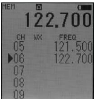
You may also overwrite an existing memory channel or select an available memory channel other than the first one displayed. Once again, select the desired frequency and then press the Memory key.
