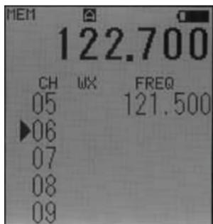
The first available memory channel will be displayed with an arrow on the screen. In this example, memory channel 06 is the first available location. To store the frequency, press the Memory key a second time. The screen will now display the following for one second to verify 122.700 has been stored in memory channel 06.
