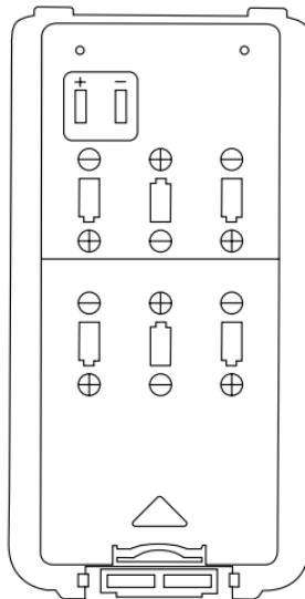
Replace the batteries by following the positive (+) and negative (-) terminal markings inside the case. When the batteries are replaced, replace the battery cover and attach the battery pack to the radio.
