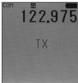
Release the PTT to end the transmission and the PJ2+ COM will once again receive the selected COM frequency. If a headset is being used, the PJ2+ COM's internal microphone will be deactivated and the microphone on the headset may be activated by either pressing the PJ2+ COM's PTT or pressing an inline remote PTT.
