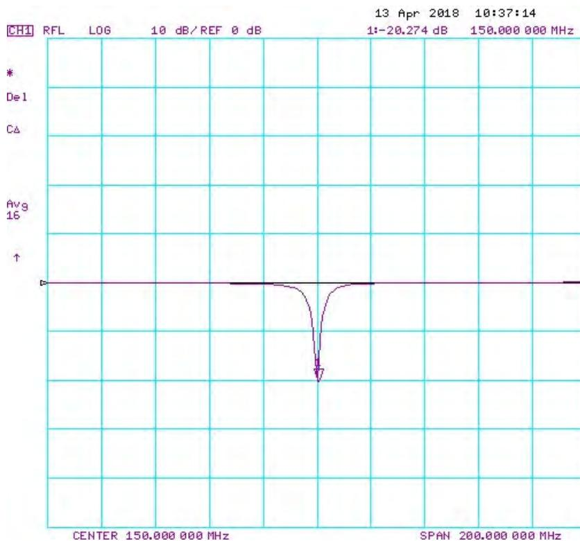
**150 MHz Dipole Extended Calibration**
