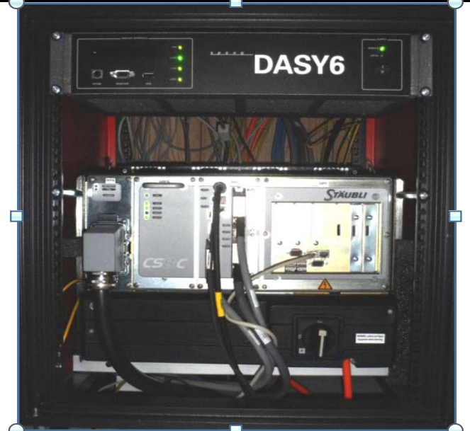
DASY 6 Measurement Controller
