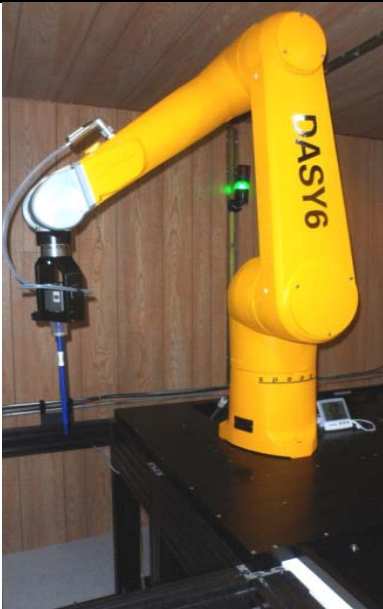
DASY 6 SAR System with SAM Phantom
