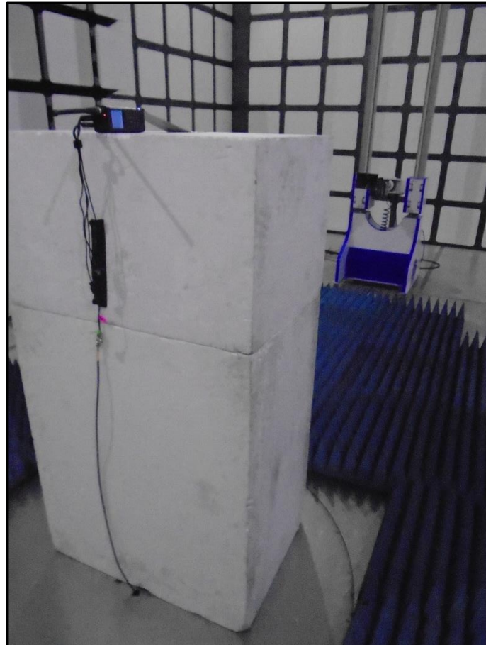
Figure 46 - Test Setup - 1 GHz to 2 GHz - Z Orientation
