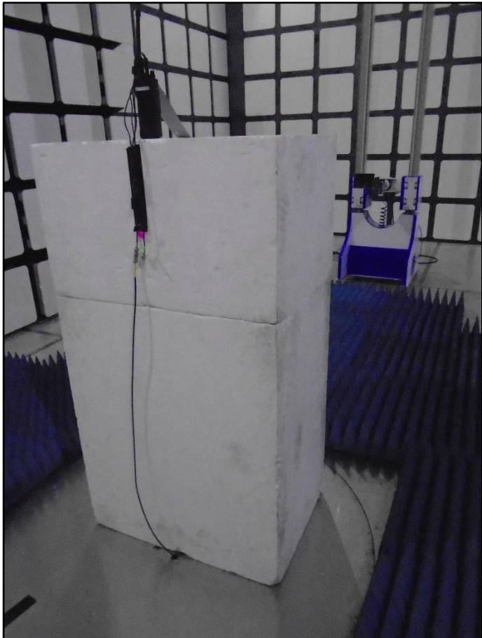
Figure 45 - Test Setup - 1 GHz to 2 GHz - Y Orientation
