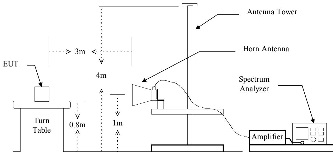
Note: For substitution method, replace the EUT with a horn antenna and connect to a standard signal generator (SG) via a low loss cable.
