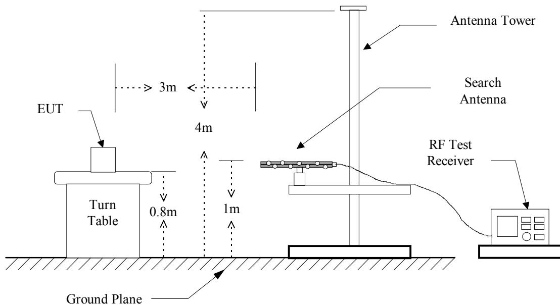
Note: For substitution method, replace the EUT with a tuned dipole antenna relative to each frequency and connect to a standard signal generator (SG) via a low loss cable.
