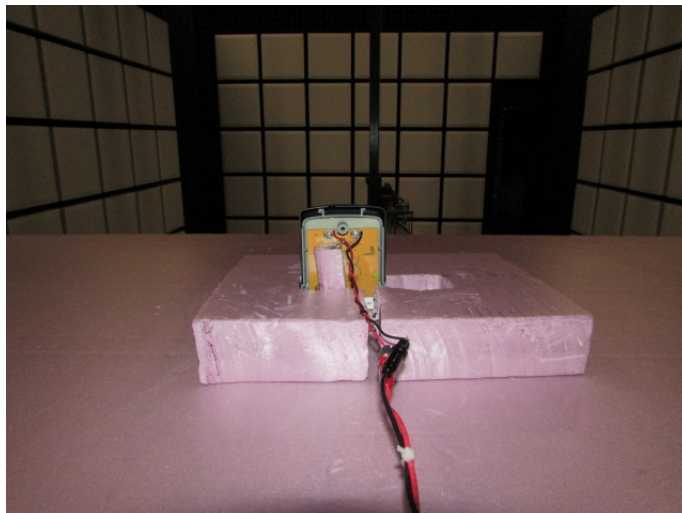
Figure 4: Radiated Spurious Emissions Test Setup – Rear View
