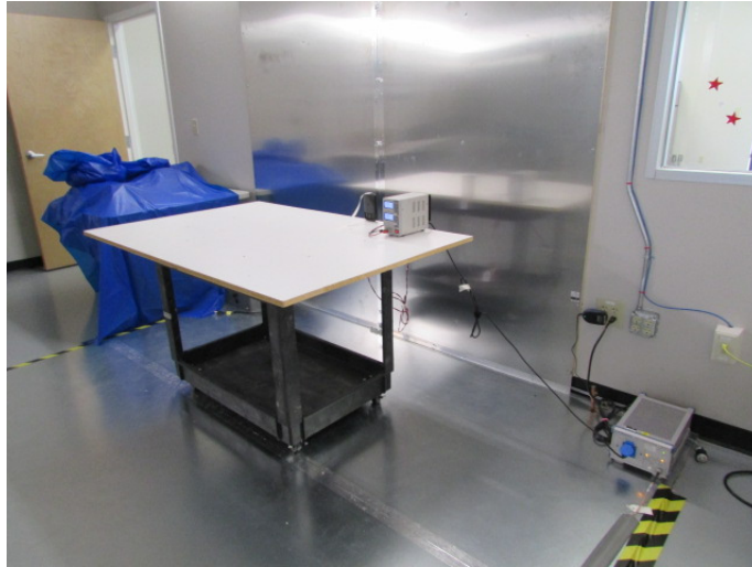
Figure 5: Power Line Conducted Test Setup – Side View
