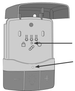
The smart wall station has two LEDs that convey information at a glance.
