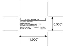
LABEL,FCC/DOC,MMT103 GTO P/N: 10015814 MFG. PROCESS: PRINTED LABEL OR PAD PRINTING LABEL INK: PERMANENT WHITE LABEL MATERIAL: CLEAR ACETATE, ADHESIVE BACKED THICKNESS: .0015" PAD PRINTING INK: WHITE (MAXCIM P/N 213337-001) SCALE: 1-1
